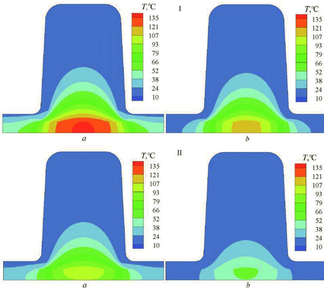
Fig. 7. Temperature fields of a polyethylene TLCPP with inner and outer diameters of 200 and 176 mm, thicknesses of the outer and inner layers of 0.8 and 1.1 mm, and an initial temperature of 160°C within 30 (a) and 60 s (b) after the beginning of the cooling: I) one-side external cooling by water with a temperature of 10°C; II) two-side cooling: external cooling by water with a temperature of 10°C and internal cooling by a water-air mixture.
