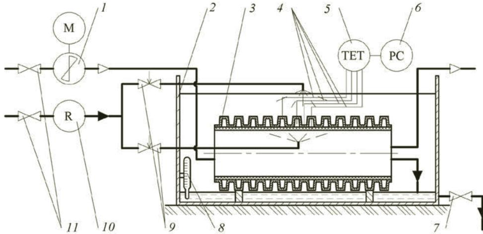
Fig. 3. Scheme of the experimental setup: 1) fan; 2) cooling vat; 3) pipe; 4) thermocouples; 5) thermoelectric temperature transducer; 6) computer; 7, 11) cocks; 8) thermometer; 9) valves; 10) rotameter.
