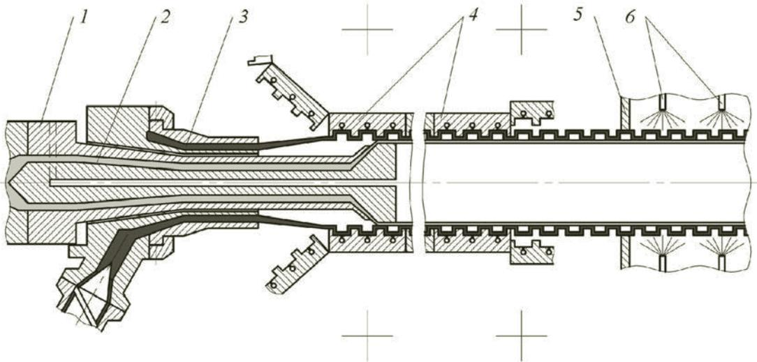
Fig. 1. Scheme of production of a TLCPP: 1) direct-flow extrusion head; 2) angular extrusion head; 3) round billet of the outer layer of the pipe; 4) half-moulds of a corrugator; 5) cooling vat; 6) injectors.
