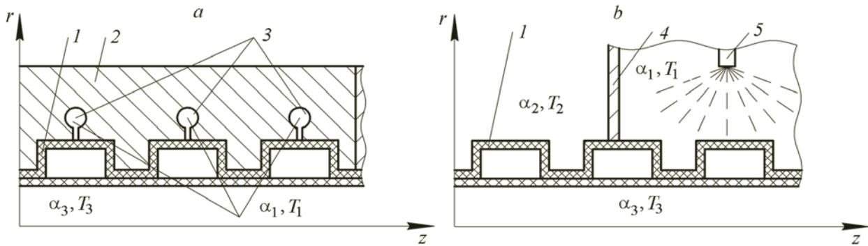
Fig. 2. Scheme of cooling of a TLCPP in a corrugator (a) and in a cooling vat (b): 1) pipe; 2) half-mould of the corrugator; 3) channels for cooling water; 4) cooling vat; 5) injector.
