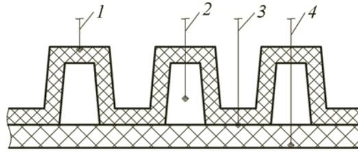
Fig. 4. Scheme of disposition of thermocouples (1–4) in the wall of a pipe.
