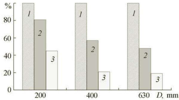
Fig. 6. Results of numerical simulation of the efficiency of cooling of pipes different in diameter for a definite period of time depending on the cooling method: 1) one-side external cooling by water; 2) two-side cooling: external cooling by water and internal cooling by air; 3) two-side cooling: external cooling by water and internal cooling by a water-air mixture.
