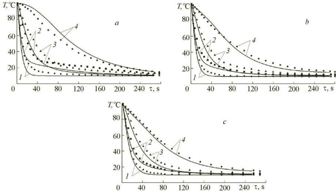
Fig. 5. Temperature fields in the wall of a pipe in the case of external water cooling (a) and two-side cooling: external cooling by water and internal cooling by air (b) and external cooling by water and internal cooling by a water-air mixture (c): 1–4, numbers of thermocouples as in Fig. 4; points, experimental data; lines, calculation.
