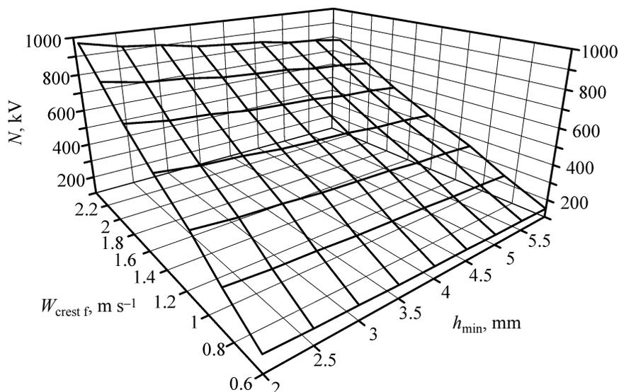
Fig. 4. The dependence of the drive power of the mixer on the depth of the minimum gap and speed of rotation of the fast rotor.
