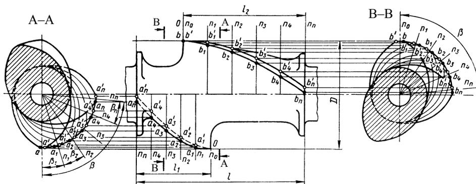
**Fig. 2.** Construction of a profile of the working part of the mixer rotor [1]:  $(n_i, \beta_i, a_i, b_i)$  beams, central angles, points and their projections, respectively.
