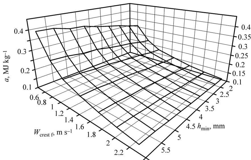
Fig. 6. The dependence of the specific mixing work on the depth of the minimum gap and speed of rotation of the fast rotor.
