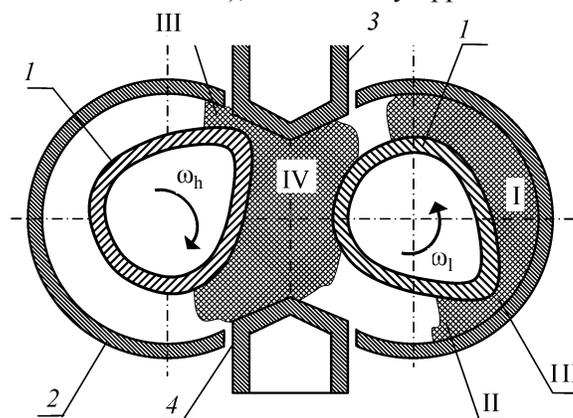
**Fig. 1.** Scheme of processing the composition in the mixer chamber. (1) Rotors; (2) operation chamber; (3, 4) upper and lower closures; (I–VI) characteristic regions of strain mixtures; ( $\omega_h$ ) and ( $\omega_l$ ) angular velocity of a high-speed and low speed rotors, rad/s.
