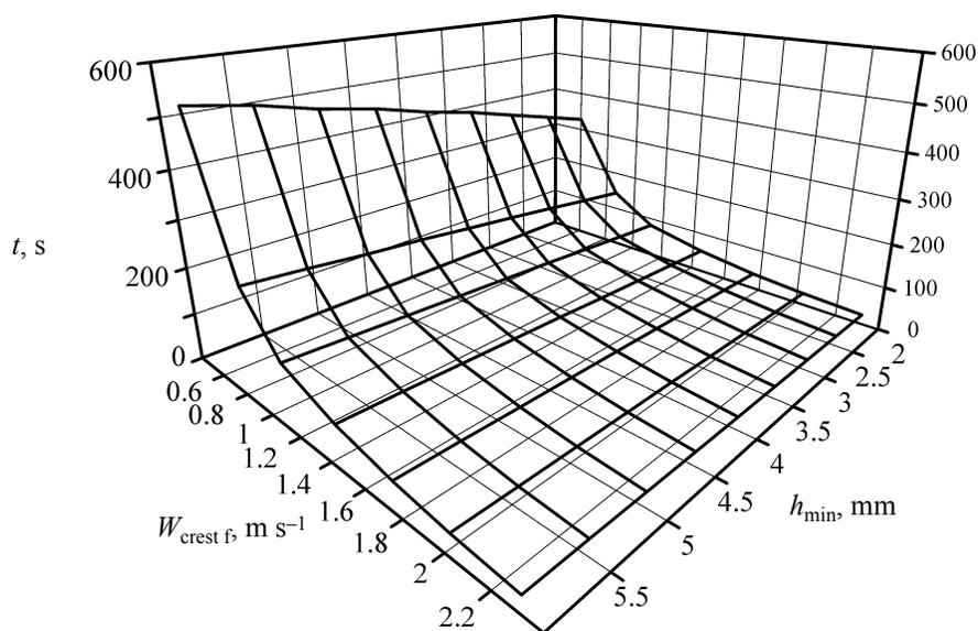
Fig. 5. The dependence of the mixing time on the depth of the minimum gap and speed of rotation of the fast rotor.
