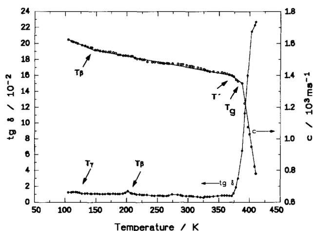
Figure 2 Temperature dependence of loss tangent and velocity of sound for annealed PPS
