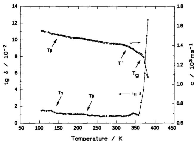
Figure 1 Temperature dependence of loss tangent and velocity of sound for amorphous PPS
