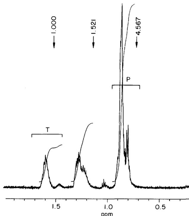
**Figure 3** <sup>1</sup>H n.m.r. spectrum of the propene oligomers soluble in boiling methanol. Propene = 7 dm<sup>3</sup>, toluene = 50 cm<sup>3</sup>, [Et[IndH<sub>4</sub>]<sub>2</sub>ZrCl<sub>2</sub>] = 1.5 × 10<sup>-4</sup> mol l<sup>-1</sup>, Al/Zr = 1700, 0°C, 5 min
