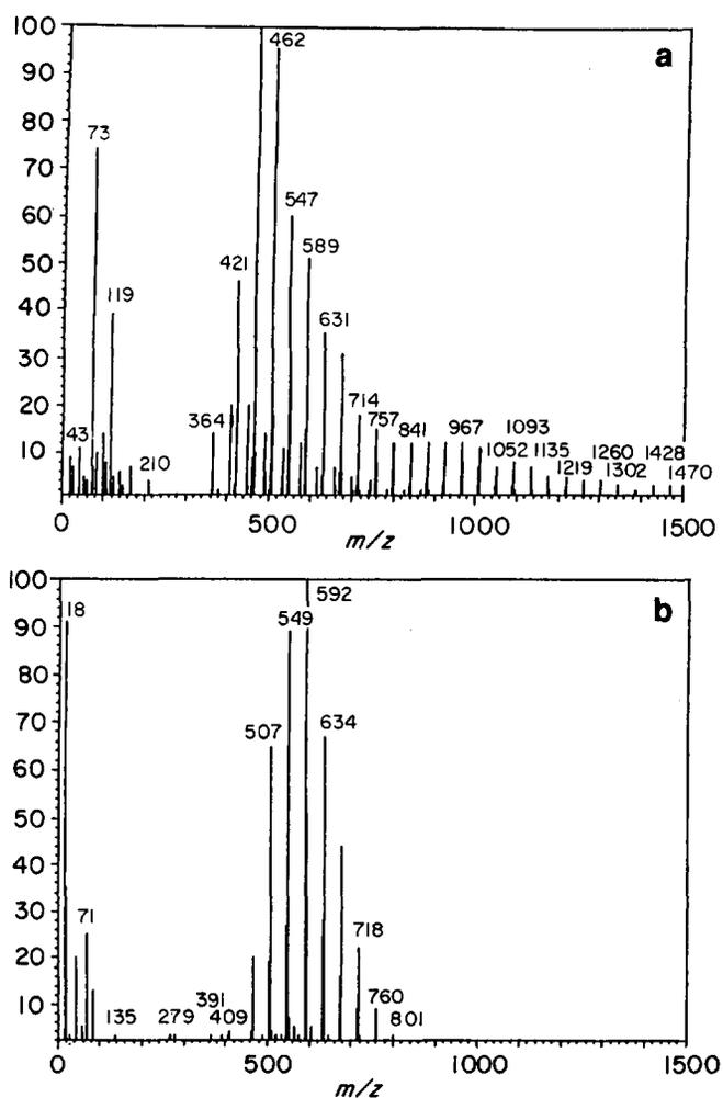
**Figure 2** Mass spectra of polypropylene. Polymerization conditions: propene = 7 dm<sup>3</sup>, toluene = 50 cm<sup>3</sup>, [catalyst] = 1.5 × 10<sup>-4</sup> mol l<sup>-1</sup>, Al/Zr = 1700, 0°C, 5 min. (a) Cp<sub>2</sub>ZrCl<sub>2</sub>/MAO catalyst; (b) Et[IndH<sub>4</sub>]<sub>2</sub>ZrCl<sub>2</sub>/MAO catalyst
