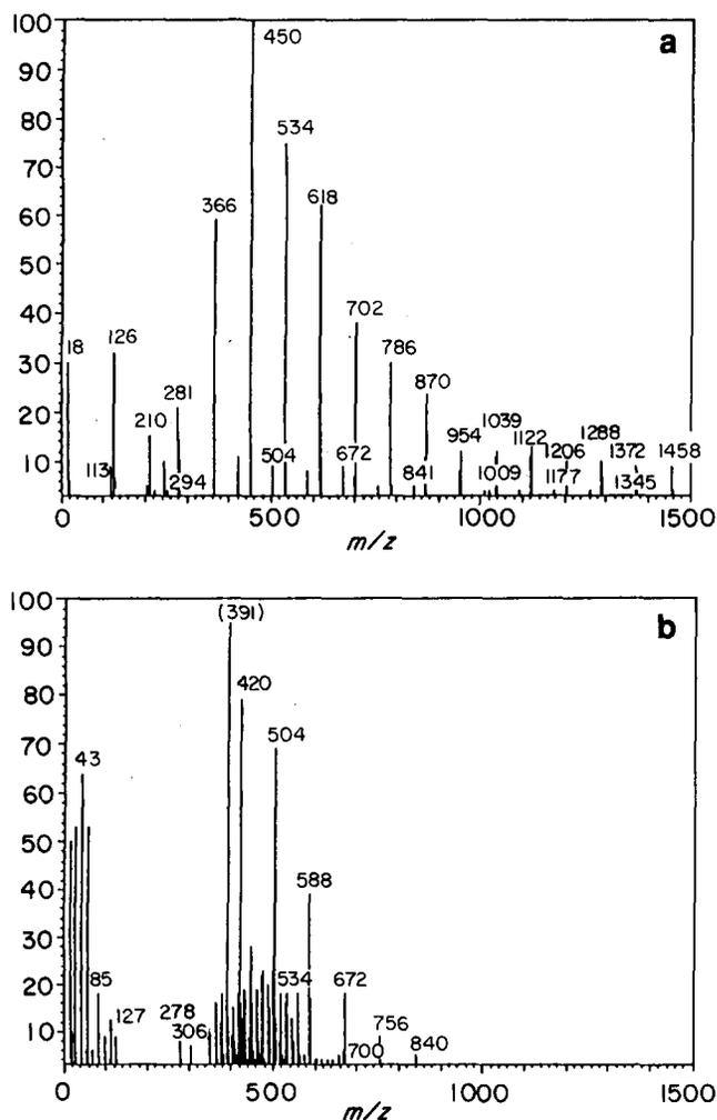
**Figure 1** Mass spectra of poly(1-hexene). Polymerization conditions: [1-hexene] = 0.2 mol l<sup>-1</sup>, [cocatalyst] = 10 mmol l<sup>-1</sup>, heptane = 100 cm<sup>3</sup>, 0°C, 5 min. (a) TiCl<sub>3</sub>/MgCl<sub>2</sub> (1.26 g; 0.03 wt% Ti)/Al(C<sub>2</sub>H<sub>5</sub>)<sub>3</sub> catalyst; (b) Solvay TiCl<sub>3</sub> (0.08 g)/Cp<sub>2</sub>Ti(CH<sub>3</sub>)<sub>2</sub> catalyst
