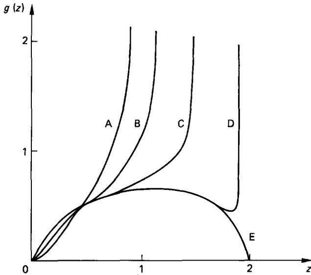
Figure 2 Distribution function of free chain ends, equation (9), in a concave cylindrical monodisperse dry layer for the values of  $r = R/H_{10}^{lam} = \infty$  (A), 3.6 (B), 2.25 (C), 2.006 (D) and 2 (E)
