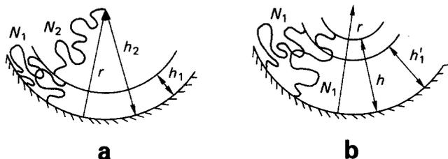
**Figure 6** Scheme for concave cylindrical layers: (a) bidisperse layer with  $r$ , cylinder radius,  $h_2$ , thickness of long-chain sublayer and  $h_1$ , thickness of short-chain sublayer; (b) monodisperse layer with  $r$ , cylinder radius,  $h_1$ , thickness of the sublayer in which the free ends of chain fraction  $q_1 = 1 - q_2$  are located and  $h$ , total layer thickness
