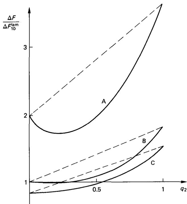
Figure 10 Relative free energy  $\Delta F/\Delta F_{10}^{\text{lam}}$  of a bidisperse layer versus  $q_2$  for (A) concave cylindrical, (B) planar and (C) convex cylindrical layers for a value of  $\alpha = 0.8$  and the radius of cylinder  $r = 2(1 + \alpha q_2)$ . ---, Dependences  $q_1 \Delta F(q_1 = 1) + q_2 \Delta F(q_2 = 1)$
