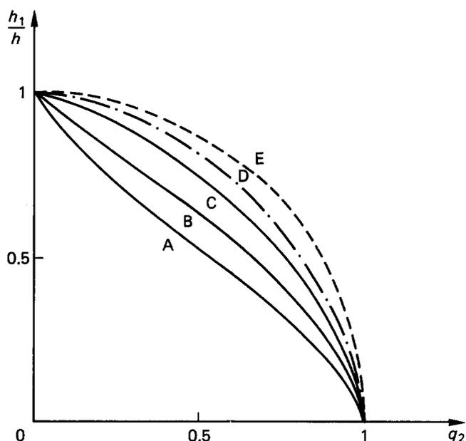
Figure 5 Ratio of the thickness  $h_1$  of a short-chain sublayer in a bidisperse layer of grafted chains to the total thickness  $h$  of monodisperse layer, equations (7), (32) and (34), versus  $q_2$  at different  $\alpha = 0$  (A), 0.1 (B), 0.86 (C),  $\infty$  (D). The asymptotic dependence  $h'_1/h$  on  $q_2$  in a monodisperse layer, equation (13) is shown in (E)
