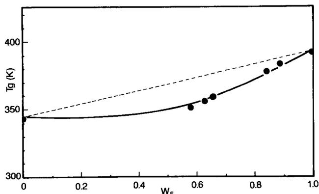
Figure 5 Glass transition temperature,  $T_g$ , of F-P copolymers as a function of the weight fraction of F,  $W_F$ , in the copolymer chains
