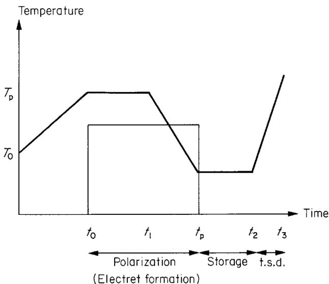
Figure 2 T.s.d. procedure represented schematically as temperature and electric field manipulations as a function of time:  $T_0$ , initial temperature;  $T_p$ , polarization temperature;  $t_0$ , start of polarization;  $t_1$ , start of cooling;  $t_p$ , time of switching off the field;  $t_2$ , start of heating;  $t_3$ , end of heating
