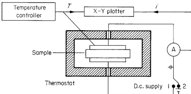
Figure 1 Schematic diagram of the t.s.d. apparatus
