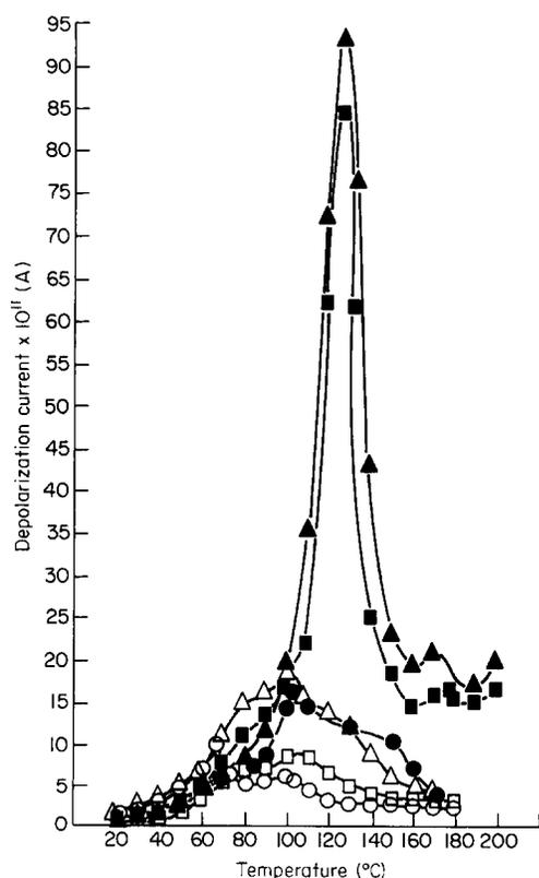
Figure 3 T.s.d. spectra of PET/0.6PHB samples polarized with a  $13.33 \text{ MV m}^{-1}$  field for several polarization temperatures: (○)  $50^\circ\text{C}$ ; (□)  $70^\circ\text{C}$ ; (△)  $90^\circ\text{C}$ ; (●)  $110^\circ\text{C}$ ; (■)  $130^\circ\text{C}$ ; (▲)  $150^\circ\text{C}$
