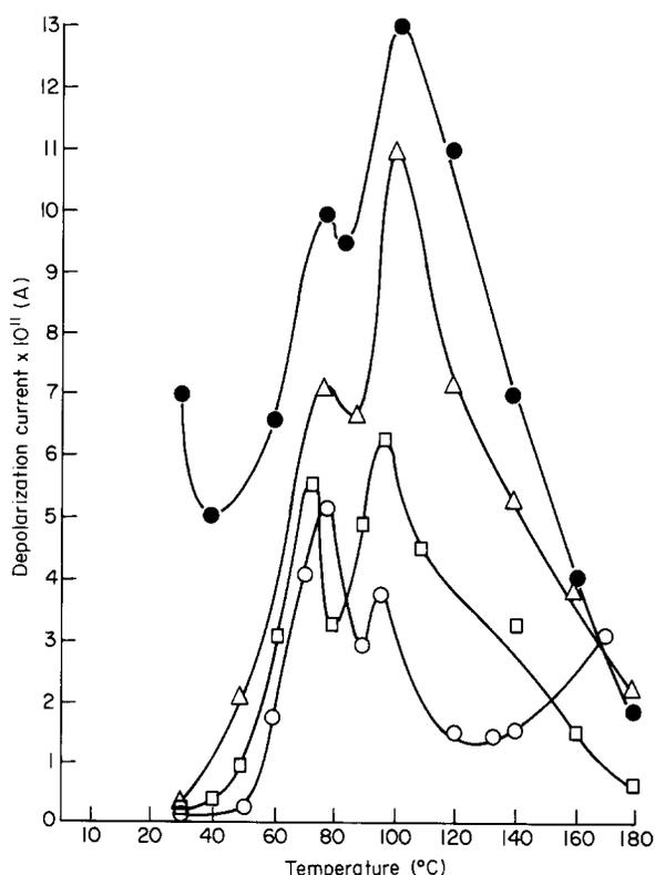
**Figure 5** T.s.d. spectra of PET/0.6PHB samples polarized at 90°C and stored for varying ageing times: (○) 125 h; (□) 25 h; (△) 5 h; (●) 0 h
