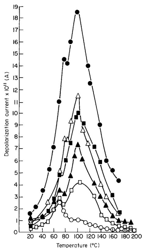
Figure 4 T.s.d. spectra of PET/0.6PHB samples polarized at  $90^\circ\text{C}$  at various electric fields: (○)  $3.33\text{ MV m}^{-1}$ ; (□)  $5.00\text{ MV m}^{-1}$ ; (△)  $6.66\text{ MV m}^{-1}$ ; (■)  $8.33\text{ MV m}^{-1}$ ; (△)  $10.00\text{ MV m}^{-1}$ ; (●)  $13.33\text{ MV m}^{-1}$
