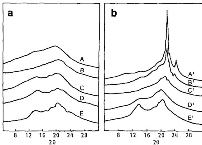
Figure 4 WAXD spectra for (a) PPO-polyether-based and (b) PBA-polyester-based PUUs: (A) ET-25-2000; (B) ET-36-2000; (C) ET-43-2000; (D) ET-50-2000; (E) ET-54-2000; (A') ES-25-2000; (B') ES-36-2000; (C') ES-43-2000; (D') ES-50-2000; (E') ES-54-2000
