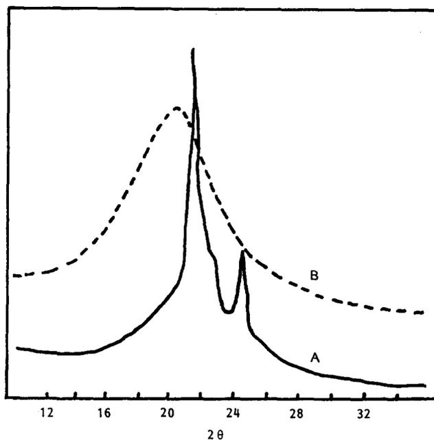
Figure 5 WAXD spectrum for ES-25-2000 at: (A) 25°C; (B) 48°C
