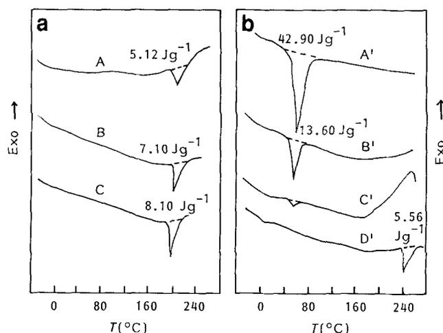
**Figure 3** D.s.c. thermograms for (a) PPO-polyether-based and (b) PBA-polyester-based PUUs: (A) ET-25-2000; (B) ET-43-2000; (C) ET-50-2000; (A') ES-25-2000; (B') ES-43-2000; (C') ES-50-2000; (D') ES-62-2000
