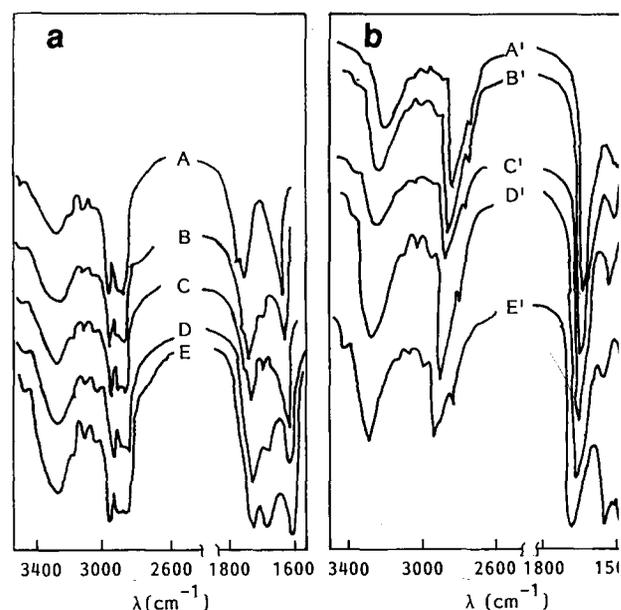
**Figure 2** I.r. spectra showing the NH and carbonyl regions for PPO-polyether-based (a) and PBA-polyester-based PUUs: (A) ET-36-2000; (B) ET-43-2000; (C) ET-50-2000; (D) ET-54-2000; (E) ET-62-2000; (A') ES-36-2000; (B') ES-43-2000; (C') ES-50-2000; (D') ES-54-2000; (E') ES-62-2000
