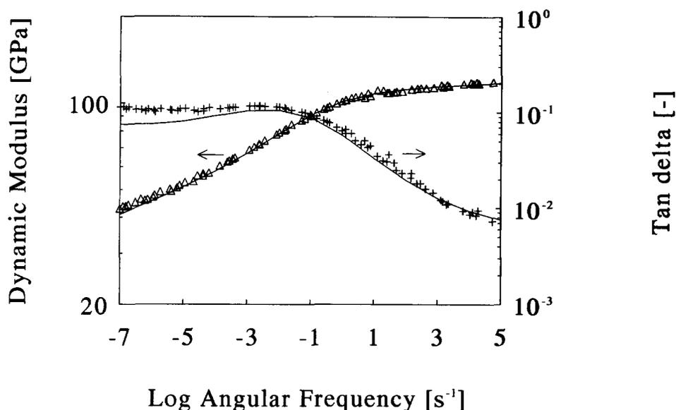
**Figure 7** Master curves of the dynamic modulus ( $\Delta$ ) and  $\tan \delta$  (+) of SK66 vs. the logarithm of the angular frequency for a reference temperature of 30°C. The full curves represent the fit obtained with the continuous relaxation-time spectrum of *Figure 9*
