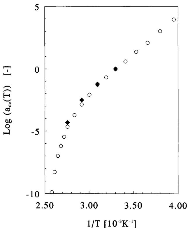
**Figure 8** Arrhenius plot of the horizontal shift factor  $a_{de}(T)$ , for a reference temperature of 30°C: (○) shift factor as derived from the dynamic quantities; (◆) shift factor as derived from stress relaxation experiments in the linear region
