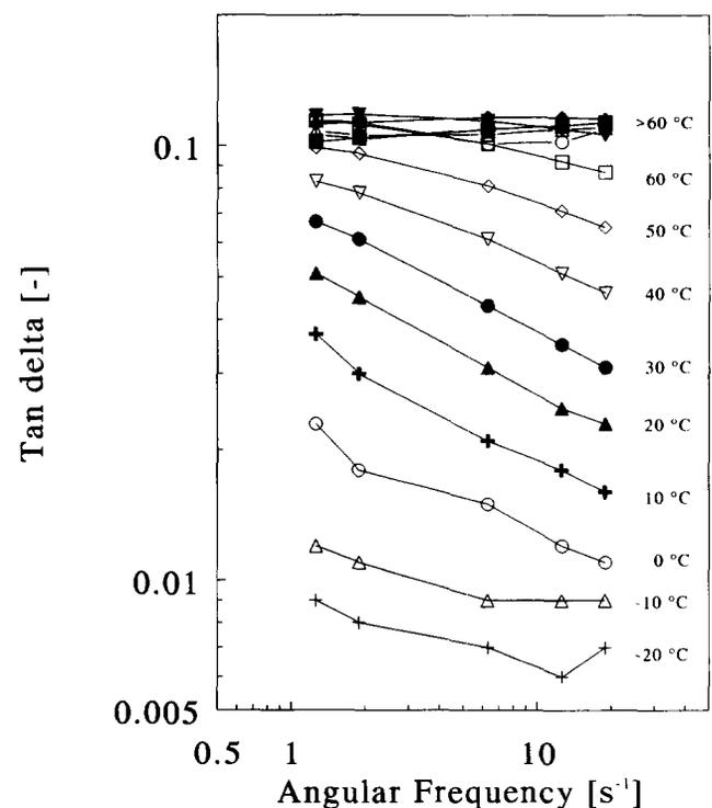
Figure 6  $\tan \delta$  of SK66 vs. angular frequency at temperatures from  $-20$  to  $105^{\circ}\text{C}$
