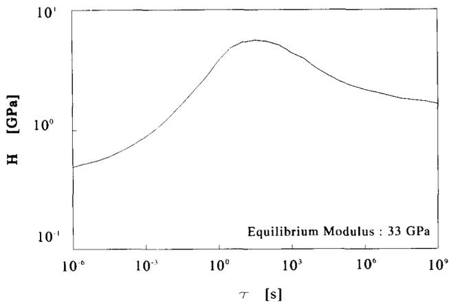
Figure 9 The continuous relaxation-time spectrum  $H(\tau)$  of SK66 for a reference temperature of 30°C
