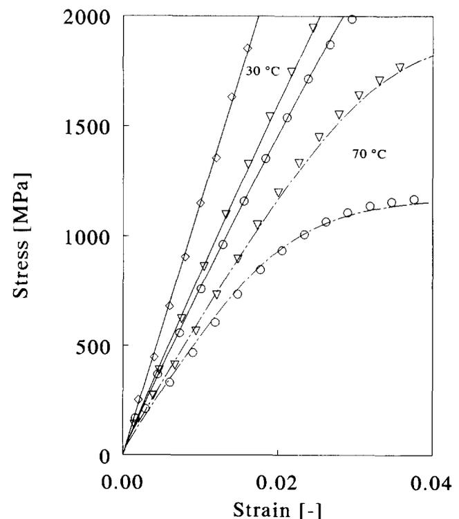
Figure 10 Constant-strain-rate experiments at various temperatures and strain rates of  $10^{-4}$  s<sup>-1</sup> (○),  $10^{-3}$  s<sup>-1</sup> (▽) and  $10$  s<sup>-1</sup> (◇), compared with model predictions (curves)
