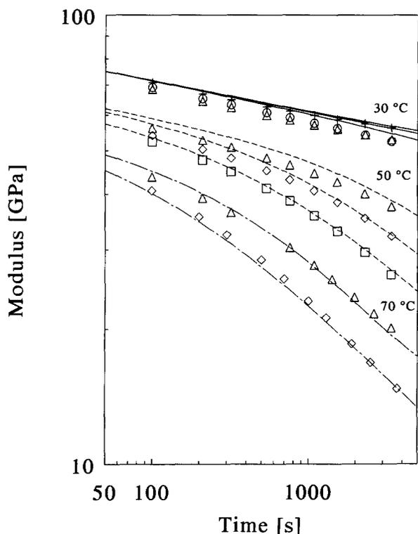
Figure 11 Stress relaxation experiments at various temperatures and strain levels of 0.5% (+), 1.0% (○), 1.5% (△), 2% (◇) and 2.5% (□), in comparison with model predictions (curves)
