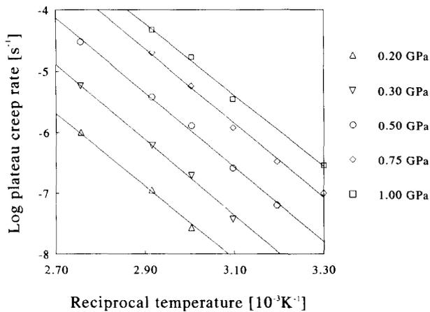
Figure 4 Arrhenius plots of the plateau creep rate at various stresses
