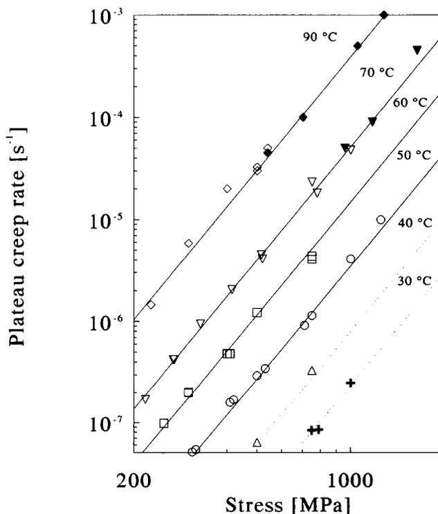
**Figure 3** Stress dependence of the plateau creep rate at temperatures of 30°C (+), 40°C ( $\Delta$ ), 50°C ( $\circ$ ), 60°C ( $\square$ ), 70°C ( $\nabla$ ) and 90°C ( $\diamond$ ). The symbols ( $\blacktriangledown$ ) and ( $\blacklozenge$ ) represent data obtained by constant-strain-rate experiments
