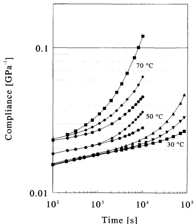
Figure 1 Creep compliance of UHMW-PE yarn (SK66) at various temperature and loads: 250 MPa (●), 400 MPa (◆), 500 MPa (■), 750 MPa (▼) and 1 GPa (▲)
