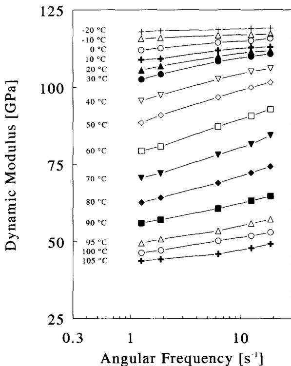
Figure 5 Dynamic modulus of SK66 vs. angular frequency at temperatures from  $-20$  to  $105^{\circ}\text{C}$
