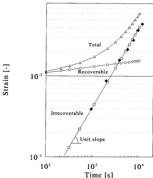
**Figure 2** Creep deformation at 70°C and a load of 500 MPa ( $\Delta$ ), decomposed into its recoverable, delayed elastic ( $\circ$ ) and irrecoverable, plastic flow ( $\square$ ) components. Experimental data on irrecoverable deformation are also represented ( $\blacklozenge$ )
