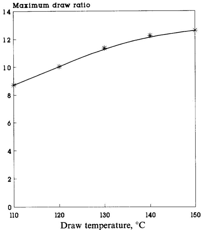
Figure 1 Maximum draw ratio vs. drawing temperature
