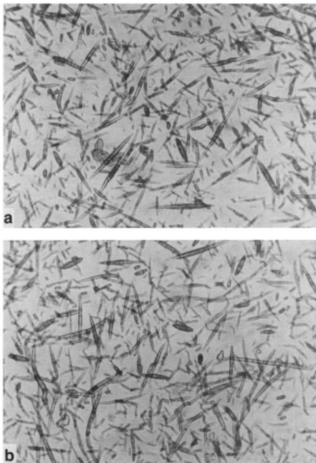
Figure 5 LCP phases of two-stage fully drawn fibres: (a) at a second-stage drawing temperature of 130°C; (b) at 160°C
