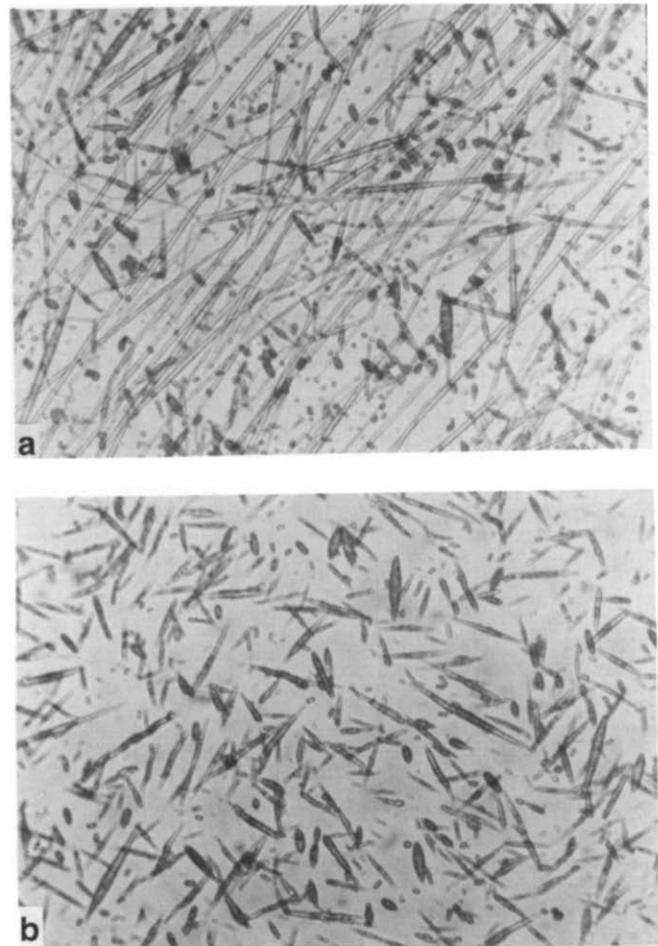
Figure 3 Hot-stage photomicrographs of the PP/LCP polyblend fibres: (a) as-spun; (b) one-stage fully drawn at 150°C
