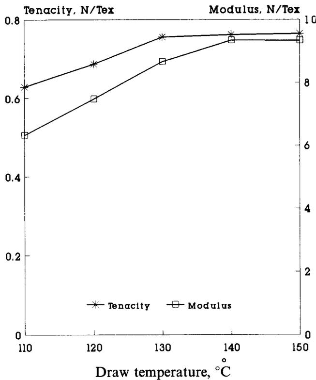
Figure 2 Fibre tenacity and initial modulus vs. drawing temperature
