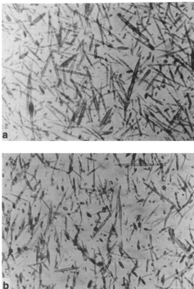
Figure 4 LCP phases from one-stage drawn fibres: (a) to a ratio of 6 at 120°C; (b) to a ratio of 10.0
