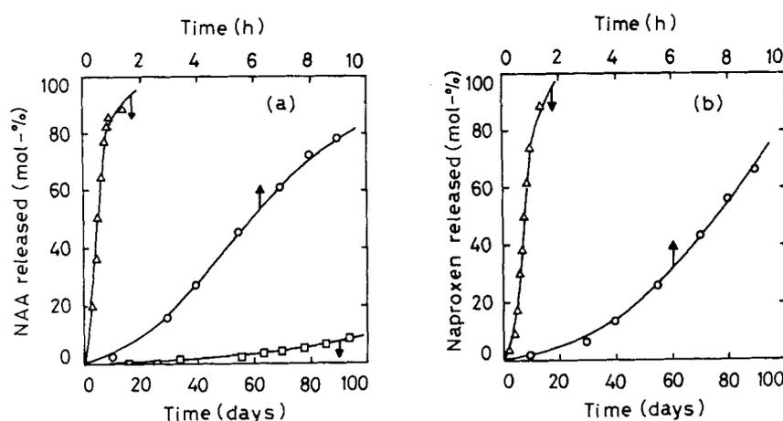
**Figure 2** Heterogeneous hydrolysis at 37°C and pH 9.0 of (a) dextran- $\alpha$ -naphthylacetic adducts with  $DS$  equal to: (○) 0.64; ( $\Delta$ ) 1.22; (□) 2.05 and (b) dextran-naproxen adducts with  $DS$  equal to: (○) 0.64; ( $\Delta$ ) 1.14
