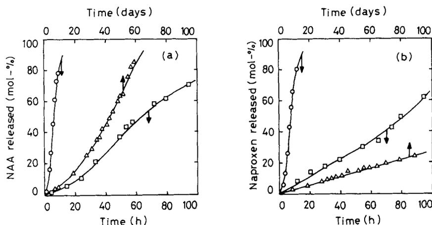
**Figure 1** Heterogeneous hydrolysis at 37°C of (a) a dextran- $\alpha$ -naphthylacetic adduct ( $DS=0.64$ ) and (b) a dextran-naproxen adduct ( $DS=0.64$ ) at various pH values: (○) 9.0; (□) 8.1; ( $\Delta$ ) 1.0. NAA =  $\alpha$ -naphthylacetic acid
