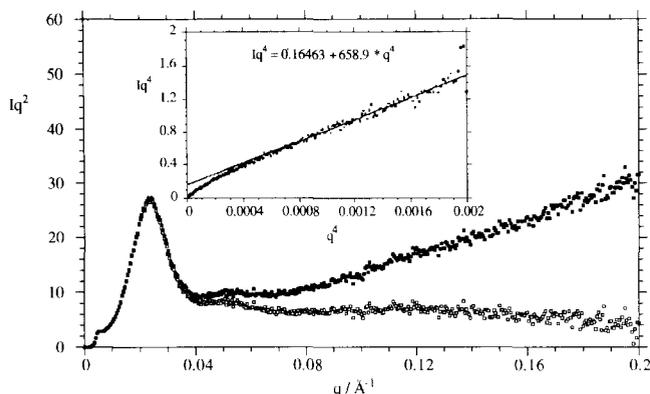
**Figure 3** Lorentz-corrected SAXS patterns at 100°C. The effects of diffuse scattering from the thermal background at high  $q$  are obvious in the raw data  $I(q)q^2$  versus  $q$  (■) and their corrected values  $[I(q) - I_b]q^2$  versus  $q$  (□). The inset is the Porod plot used to calculate the thermal background from the slope of the linear portion in  $I(q)q^4$  versus  $q^4$
