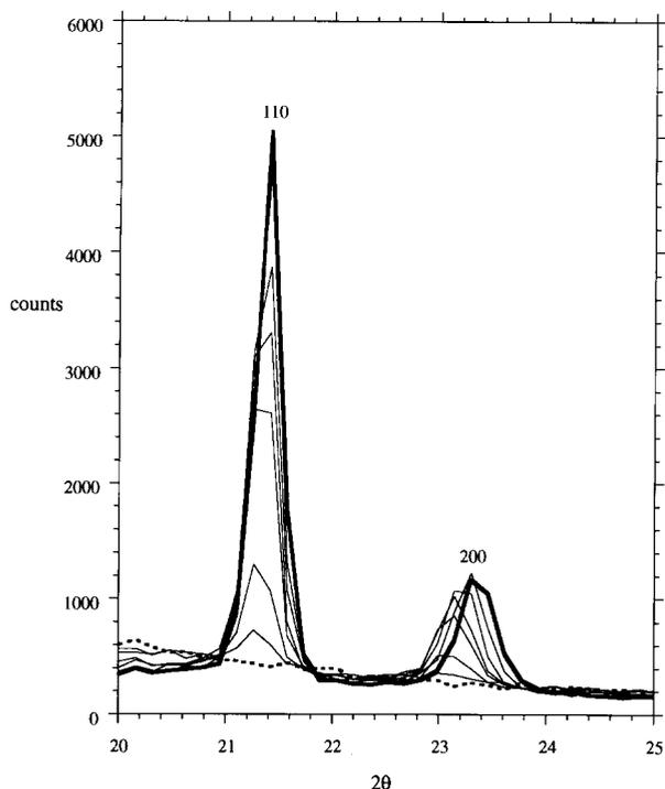
**Figure 5** Temperature dependence of the 110 and 200 regions of the WAXS patterns during melting. The thick solid curve is for 100°C and the thick dashed curve is for 160°C. The 200 peak position moves to lower  $2\theta$  as the temperature increases
