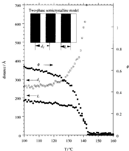
**Figure 8** The degree of crystallinity  $\phi$  ( $\blacksquare$ ) and long spacing  $d_1$  ( $\square$ ) with their product the lamellar thickness  $L$  ( $\bullet$ ) plotted as a function of temperature. The relationship between the parameters is illustrated by the two-phase semicrystalline model, which is included as an inset
