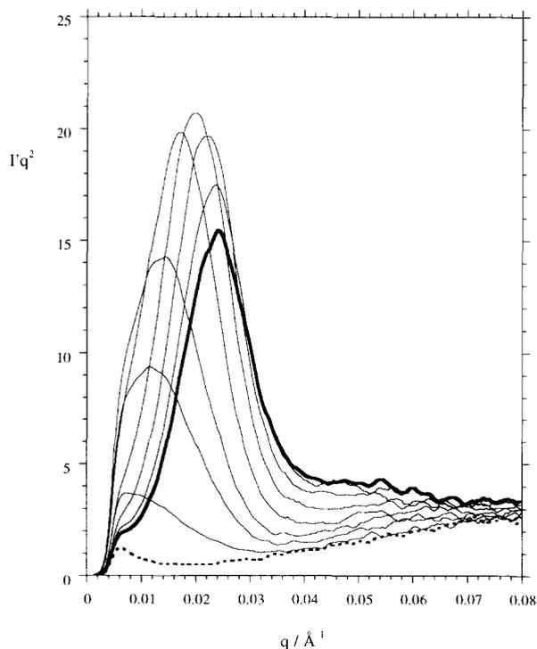
**Figure 4** Temperature dependence of the Lorentz-corrected SAXS patterns during melting. The thick solid curve is for 100 C and the thick dashed curve is for 160 C. The peak position moves towards lower  $q$  as the temperature increases
