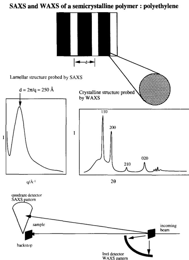
**Figure 1** Spatial information available from SAXS and WAXS experiments on semicrystalline polymers. The SAXS experiments allow calculation of the lamellar spacing from the peak maximum. The crystal structure may be deduced from the positions of the peaks in the WAXS pattern. The camera geometry is also shown
