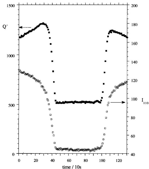
**Figure 6** Time dependence of the SAXS invariant  $Q'$  (■) and integrated WAXS intensity  $I_{110}$  (□) during melting and recrystallization of HDPE
