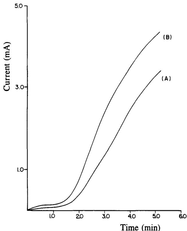
**Figure 1** Current versus time curves for the electrochemical polymerization of 0.5 M aniline at 0.7 V with 1.0 M HCl and without/with LiCl:  $[\text{LiCl}] = 0$  M (a) and 2 M (b)
