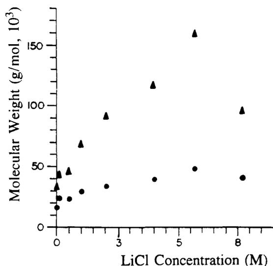
**Figure 3** Molecular weights  $M_w$  ( $\blacktriangle$ ) and  $M_n$  ( $\bullet$ ) of polyaniline as functions of the LiCl concentration used in the electropolymerization of 0.5 M aniline with 1.0 M HCl at 0.7 V and  $25^\circ\text{C}$
