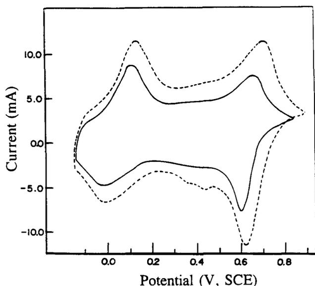
**Figure 2** Cyclic voltammogram of polyaniline electrochemically synthesized in 1.0 M HCl in (—) absence of salt and (---) presence of 2.0 M LiCl
