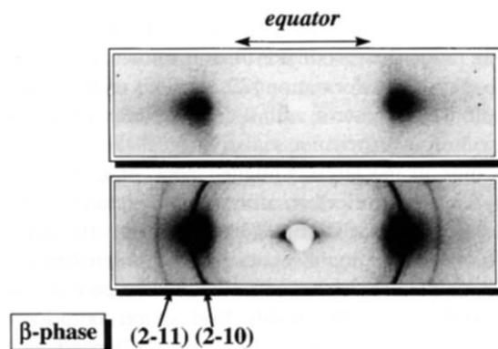
Fig. 5. Close-up of WAXS pattern recorded at (a) the centre edge of the plastic zone (pattern rotated so that equatorial scattering horizontal), and (b) 0.78 mm below centre edge of plastic zone
