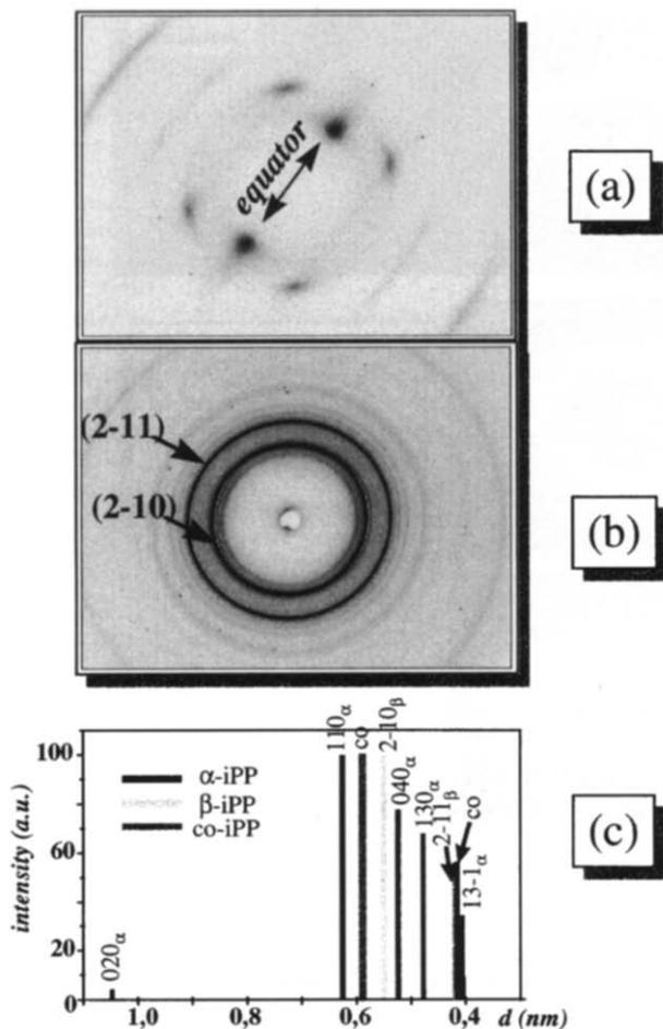
Fig. 2. WAXS pattern of (a) co-iPP recorded at centre of process zone and (b)  $\beta$ -iPP recorded in bulk zone together with Millers indices of strongest reflections. (c) Main peak positions of co-iPP,  $\alpha$ -iPP and  $\beta$ -iPP. Indexing of  $\beta$ -iPP corresponds to the trigonal P3<sub>1</sub>21 cell (hexagonal setting)[17]. Reflections of every phase scaled individually to its strongest reflection (= 100).
