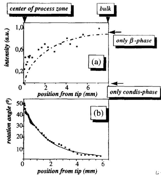
Fig. 3. (a) Variation of (2-10) reflection intensity of  $\beta$ -iPP as a function of position across the process zone. The intensity values (arbitrary units) have been scaled to 1.0 in the bulk and zero at the centre edge of the plastic zone (i.e. process zone). The line is only a guide for the eyes. (b) Variation of angle of rotation of the co-iPP equator from horizontal line. Line calculated for a first-order exponential decay.
