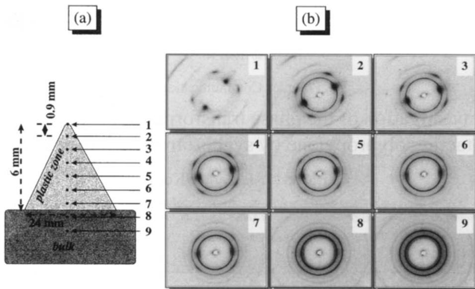
Fig. 1. (a) Schematic picture of the stress-whitened plastic zone of a DDEn-T specimen of  $\beta$ -iPP. The recording position of the WAXS patterns (1–9) are shown. Position 1 corresponds to the centre of the process zone. (b) WAXS patterns recorded at positions 1–9. Accumulation time per WAXS pattern is 1 s.
