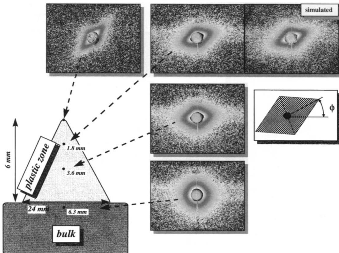
Fig. 4. SAXS patterns obtained at selected positions (logarithmic scale). Their positions are indicated relative to the first observed SAXS pattern from the process zone. The pattern at 1.8 mm was simulated by adding the patterns at 0 and 6.3 mm and rotating the summed pattern by  $\phi = 25^\circ$ .
