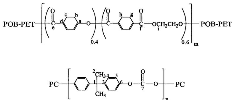
Fig. 1. The chemical structures of copoly(oxybenzoate-ethylene terephthalate) and polycarbonate.
