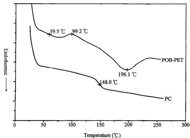
Fig. 2. The d.s.c. curves of copoly(oxybenzoate-ethylene terephthalate) and polycarbonate.
