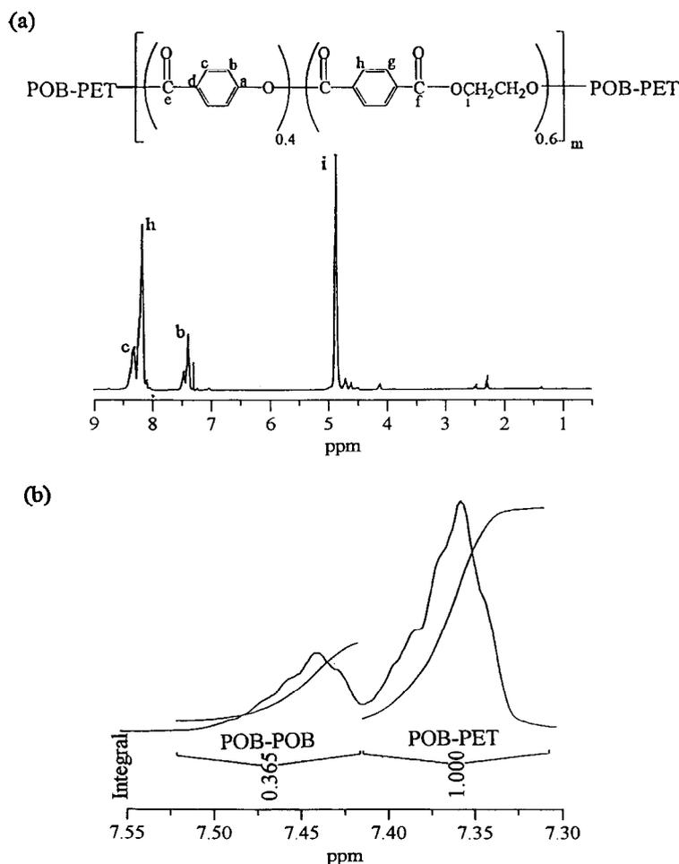
Fig. 5. (a) The full <sup>1</sup>H n.m.r. spectra of POB-PET, (b) the enlarged section of peak b in the full <sup>1</sup>H n.m.r. spectra of POB-PET.
