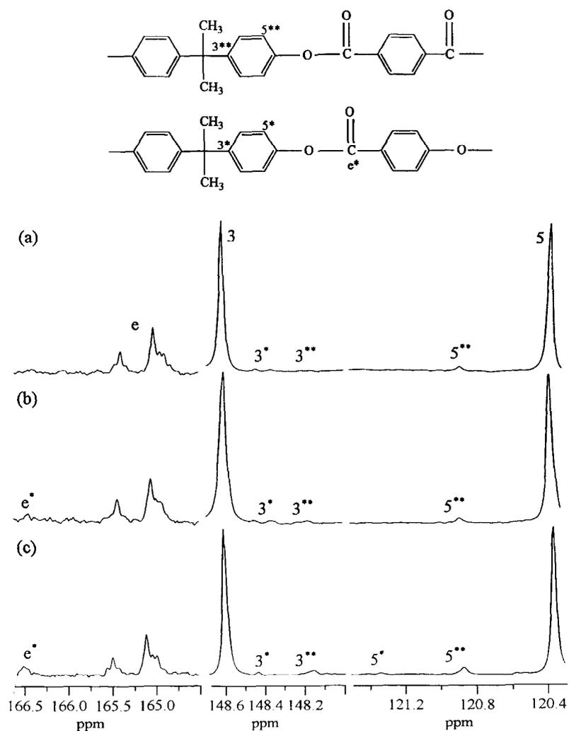
Fig. 4. The partial  $^{13}\text{C}$  n.m.r. spectra of the 60/40 POB–PET/PC blend annealed at  $250^\circ\text{C}$  for (a) 15 min, (b) 30 min, (c) 60 min.
