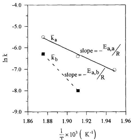
Fig. 9. The change in the rate constants  $\bar{k}_a$  and  $\bar{k}_b$  of transesterification in the 60/40 POB-PET/PC blend with the annealing temperature.
