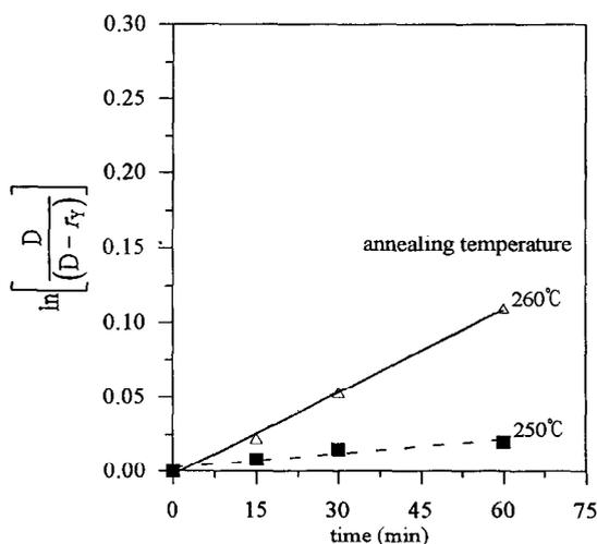
Fig. 8. The plot of the kinetic expression of dyad bisphenol A-oxybenzoate against the annealing time at different temperatures.
