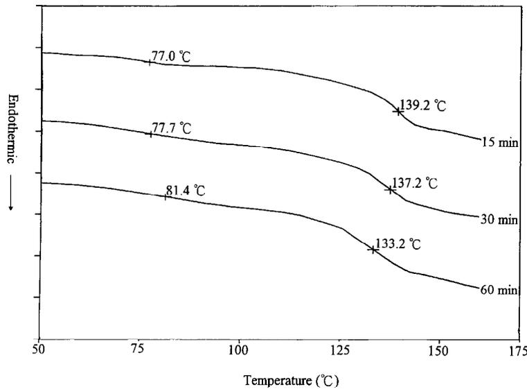
Fig. 3. The partial d.s.c. curves of the 60/40 POB–PET/PC blend annealed at 250°C for different times.
