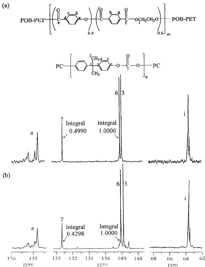
Fig. 6. The partial  $^{13}\text{C}$  n.m.r. spectra of (a) fresh 60/40 POB-PET/PC blend, (b) 60/40 POB-PET/PC blend annealed at  $260^\circ\text{C}$  for 60 min.
