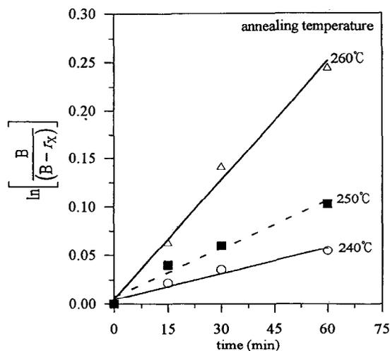
Fig. 7. The plot of the kinetic expression of dyad bisphenol A-terephthalate against the annealing time at different temperatures.
