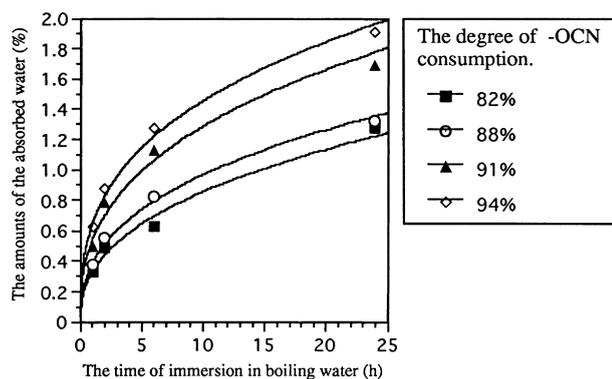
Fig. 5. Behaviour of the water pick-up rate of cured resins.
