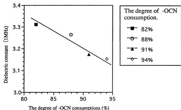
Fig. 4. Dielectric constants of cured resins having different degree of -OCN consumptions.
