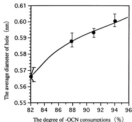
Fig. 2. Relationship between the average diameter of holes and the degree of -OCN consumption.
