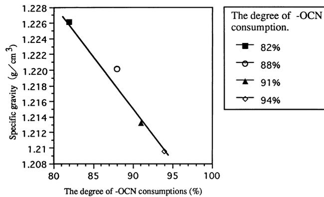
Fig. 3. Changes in the specific gravity of cured resins during a curing reaction in catalytic systems.
