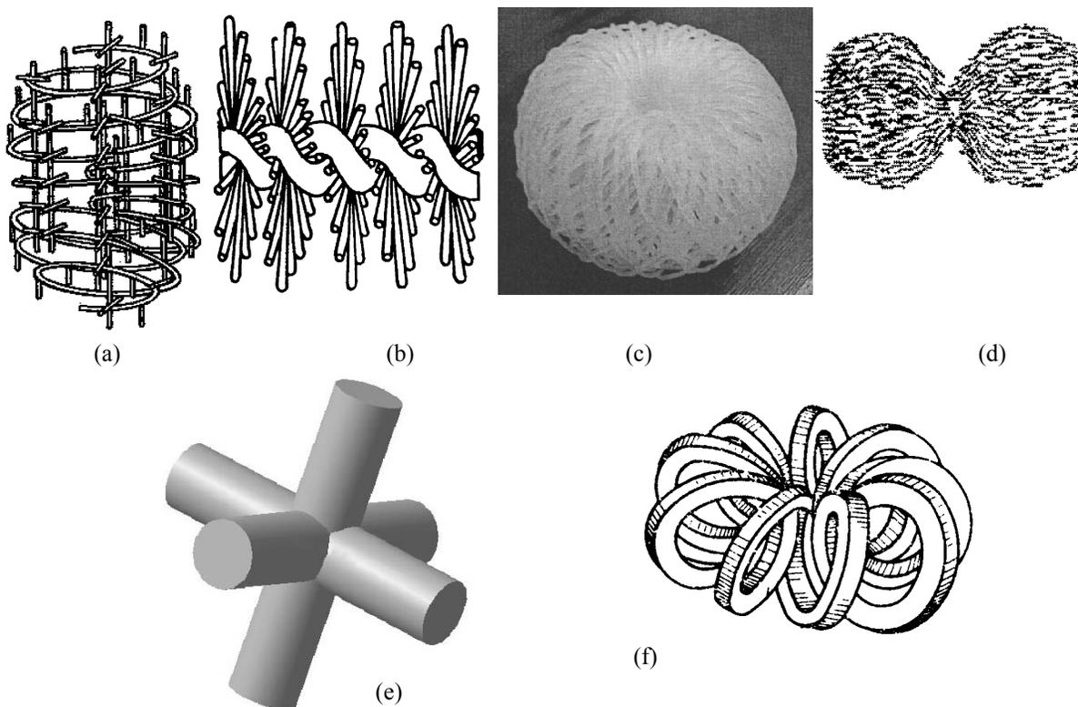
**Fig. 8.** Construction of nozzle from wire (filament) material: (a) Patent no. 5714097 US; (b) SU Inventor's Certificate no. 1669533; (c) RF Patent no. 2289472; (d) US Patent no. 5587239; (e) UA Patent no. 23562; (f) Teller socket [9].
