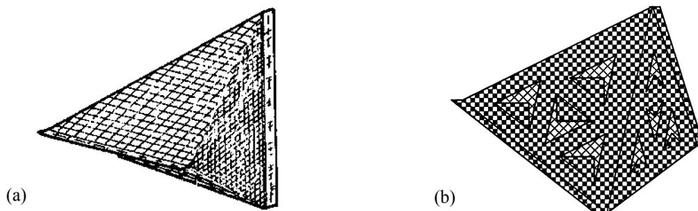
Fig. 6. Construction of nozzle in a form of reticular tetrahedron: (a) US Patent no. 6251227; (b) UA Patent no. 25414.
