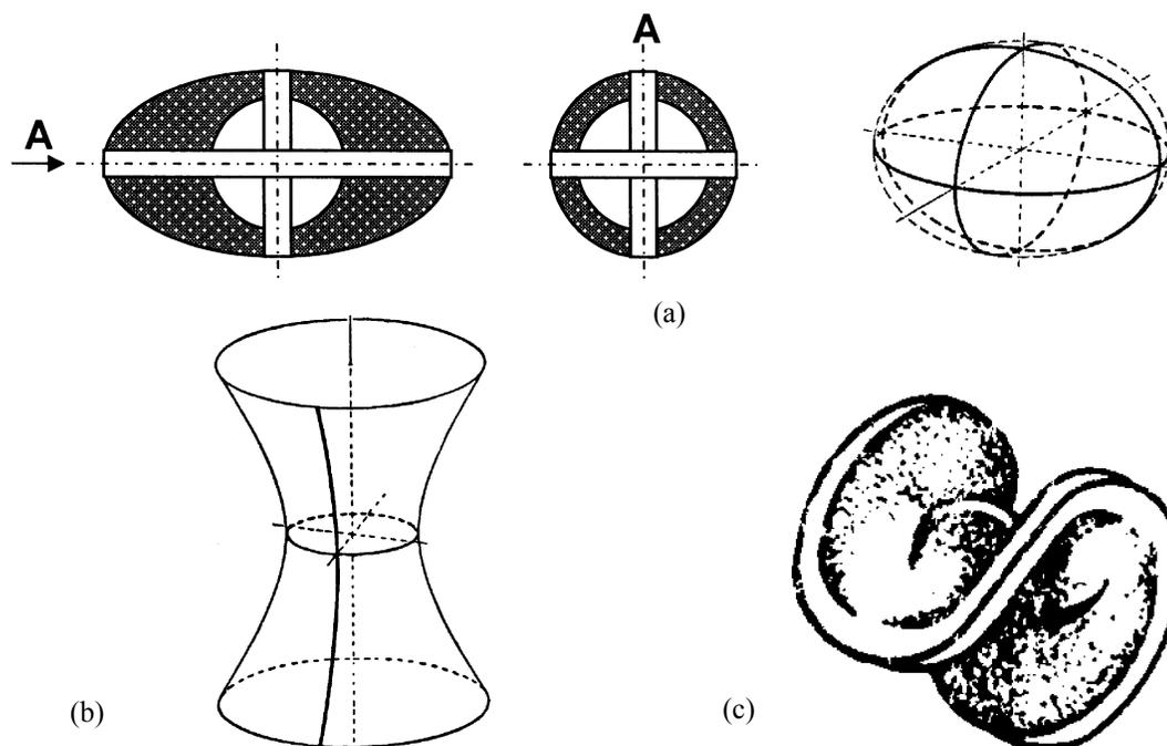
Fig. 7. Construction of nozzle in form of surfaces of second order: (a) ellipsoid (UA Patent no. 42587); (b) one-sheet hyperboloid (UA Patent no. 2396, UA Patent no. 6504); (c) hyperbolic paraboloid (Burley saddle [9]).
