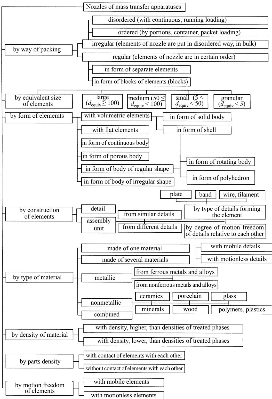
Fig. 1. Scheme of classification of nozzles of mass transfer apparatuses.
