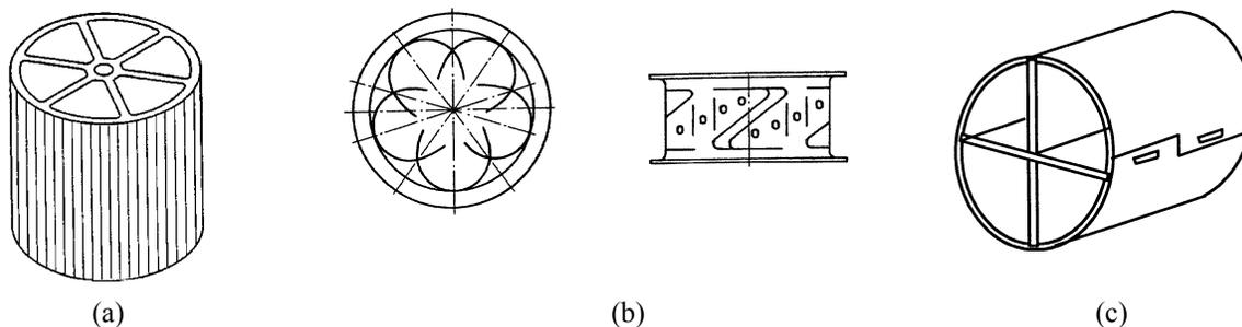
**Fig. 4.** Construction of tubular nozzle: (a) US Patent no. 5730916; (b) Nazim ring (RF Patent no. 20027504); (c) UA Patent no. 28581.
