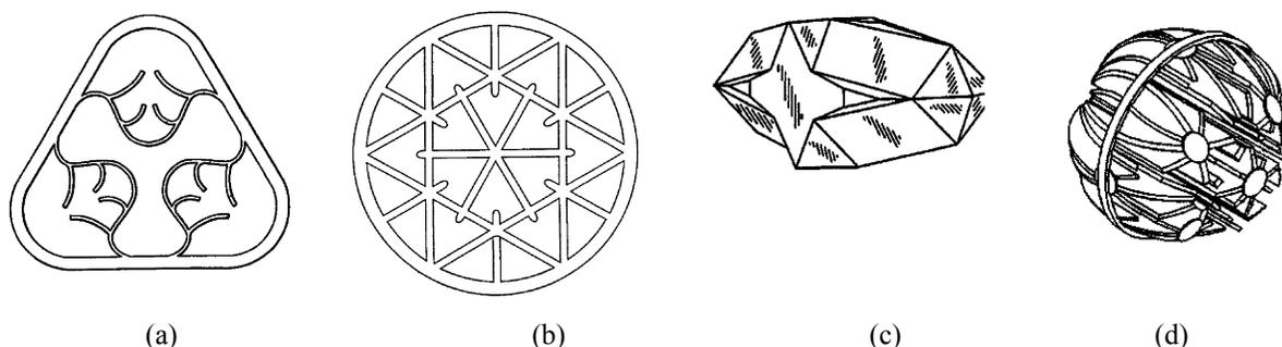
**Fig. 10.** Construction of nozzles from polymer materials: (a) WO Appl. no. 9804343; (b) RF Patent no. 2207902; (c) WO Appl. no. 9640432; (d) US Patent no. 5690819.
