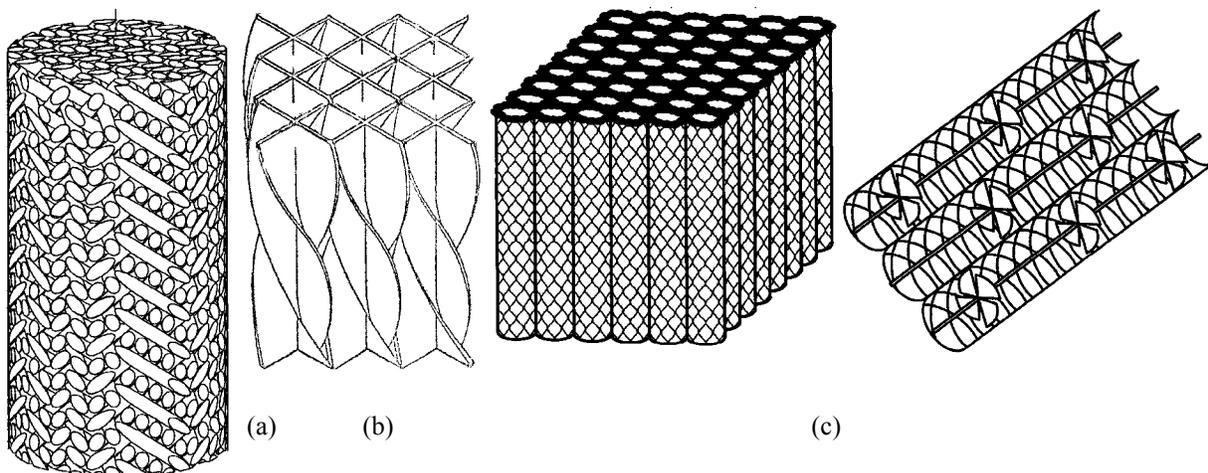
Fig. 2. Regular nozzle according to (a) RF Patent no. 2397806, (b) RF Patent no. 2350877, (c) RF Patent 2335724.
