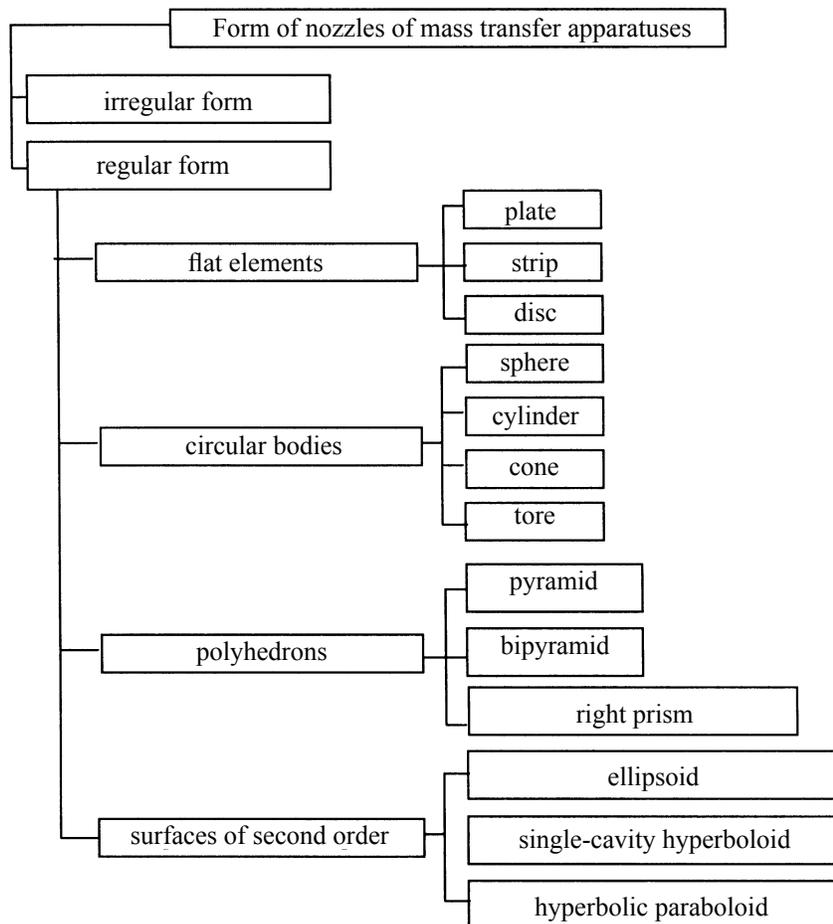
Fig. 3. Scheme of classification of nozzles by geometry.
