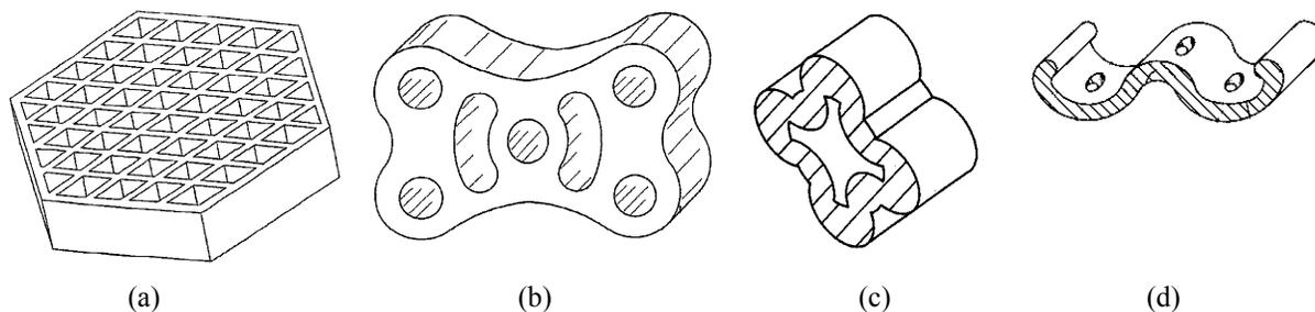
**Fig. 9.** Construction of nozzles from ceramic materials: (a) RF Patent no. 2288778; (b) RF Patent no. 2281156; (c) EP Appl. no. 0579234; (d) US Patent no. 5747143.
