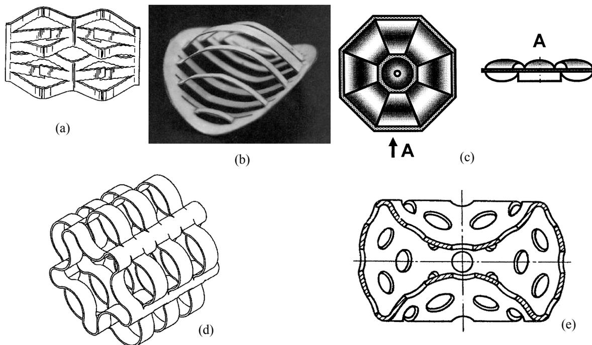
**Fig. 5.** Construction of nozzles produced from thin sheet, tubular and spherical workpieces: (a) US Patent no. 5543088; (b) RF Patent no. 2398627; (c) UA Patent no. 25416; (d) RF Patent no. 2290992; (e) SU Patent no. 1064962.
