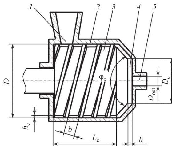
**Fig. 1.** Scheme of the disk extruder: (1) feeding inlet; (2) body; (3) disk; (4) disk gap; (5) central outlet of the body; ( $D$ ,  $D_e$ ,  $D_{out}$ ) diameters of cylindrical and end parts of the disk, and also of the central outlet of the body, respectively, m; ( $L_c$ ,  $b$ ,  $h_c$ ) length, width, and depth of the screw thread of the cylindrical part of the disk, m; ( $h$ ) size of the disk gap, m; ( $\varphi_c$ ) angle of taper of the end part of disk, deg.
