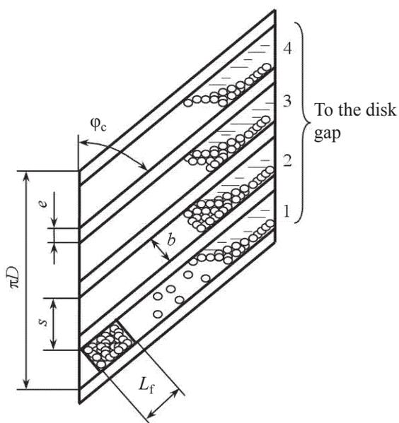
**Fig. 2.** Scheme of the four start ( $k = 4$ ) screw thread of the disk deployed on the surface: ( $s$ ,  $e$ ,  $\varphi_c$ ) pitch (m), crest width (m), and flank angle (deg) of spiral thread of cylindrical disk surface; ( $L_f$ ) length of feeding inlet of the body, m; (1–4) numbers of thread coils of disk.
