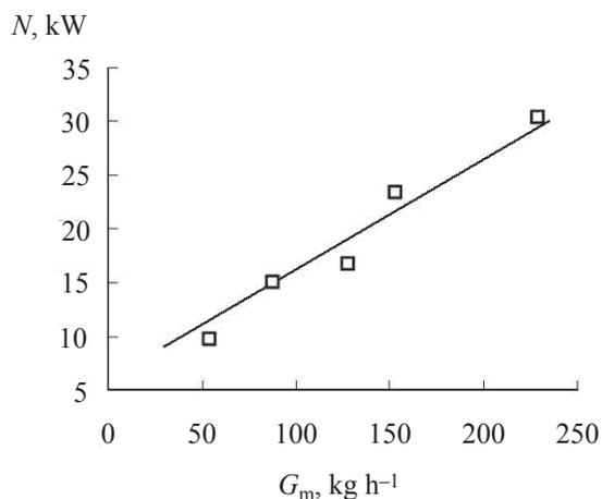
Fig. 6. The drive power of the disk extruder vs. its output.
