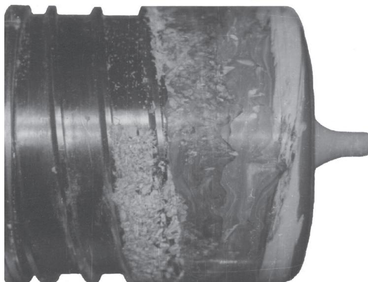
**Fig. 4.** Photograph of the disk removed from the extruder (the unmelted polymer is marked by light color).
