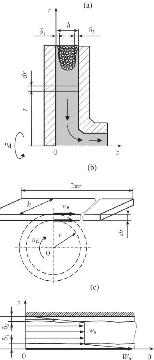
**Fig. 3.** Scheme of the process in the disk gap: (a) melting of polymer in the disk gap; (b) calculated scheme of the disk gap; (c) melt flow in the disk gap ( $W_\theta$  is the peripheral velocity of disk,  $\text{m s}^{-1}$ ;  $w_\theta$  is the peripheral component of polymer velocity in the gap,  $\text{m s}^{-1}$ ; ( $r$ ) radius of location of an elementary annular polymer volume of the width  $dr$ ,  $\text{m}$ ).
