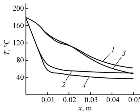
**Fig. 5.** Dependence of temperature of (1, 3) inner and (2, 4) outer surfaces of the polymer films along the cooling length  $x$ , m: (1, 2) Re = 120, (3, 4) Re = 1500.
