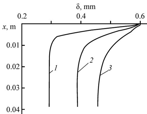
**Fig. 3.** Variation of the water film thickness along the length of the cooling zone depending on Re number : (1) 500, (2) 1000, (3) 1500.
