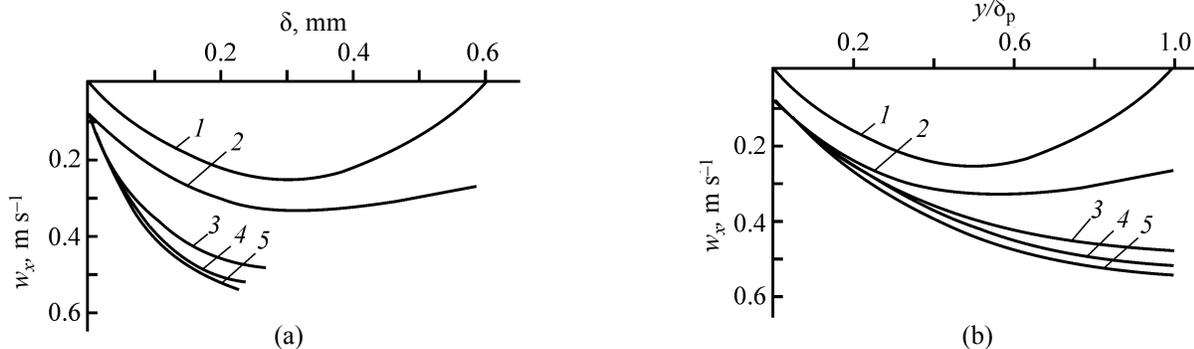
**Fig. 2.** Variation of the velocity  $w_x$  along (a) the water film thickness and (b) the dimensionless coordinate depending on coordinates  $x$ , m: (1) 0, (2) 0.005, (3) 0.03, (4) 0.045, (5) 0.06.
