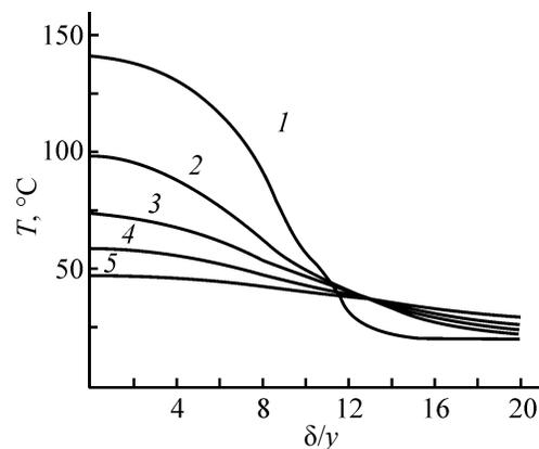
**Fig. 4.** Temperature distribution over the thickness of the polymer and fluid films depending on the coordinate  $x$ , m: (1) 0.015, (2) 0.025, (3) 0.035, (4) 0.045, (5) 0.06.
