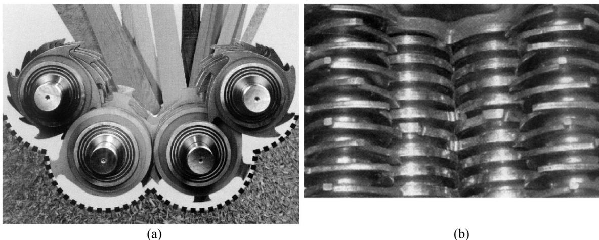
**Fig. 3.** Four rotor shredder: (a) the scheme of the operating chamber; (b) the view on rotors from the angle of the feeding bunker (Perfect technologies of crushing. Four rotor shredders series ZM 30-ZM 50: catalog, Ilsfeld (Germany): Weima Maschinenbau GmbH, [2008], p. 4).
