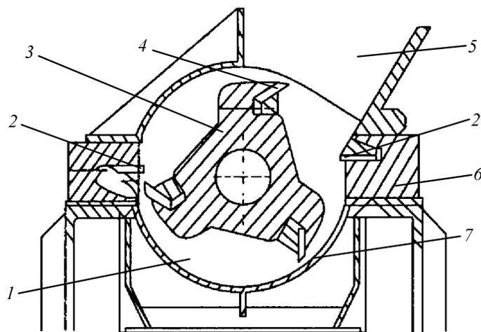
**Fig. 2.** Horizontal cutting mill: (1) the crushing chamber; (2) blades of stator; (3) the rotor; (4) blades of the rotor; (5) the feeding hole; (6) the body; (7) the sorting sieve.
