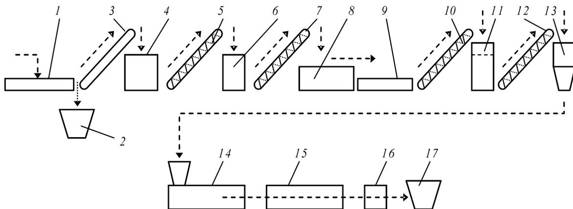
**Fig. 1.** Flow diagram of the technological production line of granulate: (1) the delivery table; (2) the bunker for impurities; (3) the band feeder; (4) the crusher; (5, 7, 10, 12) screw transporters; (6) the hot wash; (8) friction wash; (9) the flotation wash; (11) the washing device; (13) the drier; (14) the extruder; (15) the cooler; (16) the granulator; (17) the storage hopper.
