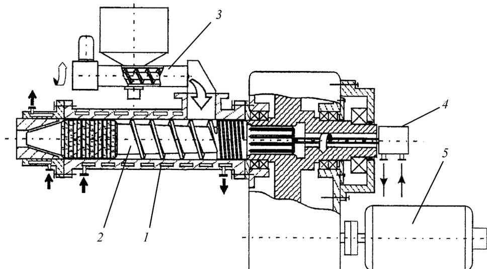
**Fig. 4.** Scheme of the construction of rotor crusher DECKCHER-150: (1) the body; (2) the rotor; (3) the dosimeter; (4) the cooling system of rotor; (5) the drive.
