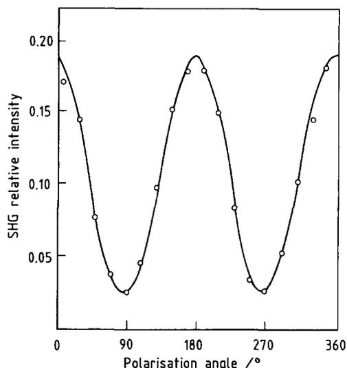
**Figure 2** SHG intensity generated from a  $6 \mu\text{m}$  film of PHIC cast under a field of  $266 \text{ V mm}^{-1}$  as a function of polarization angle
