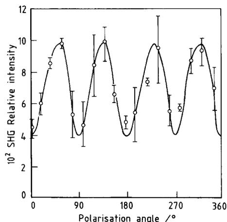
**Figure 4** SHG intensity generated from a  $20 \mu\text{m}$  film of PBLG cast under a field of  $300 \text{ V mm}^{-1}$  as a function of polarization angle
