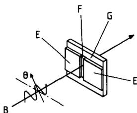
**Figure 1** Film assembly in its vertical position in the laser beam (B) showing the polarization angle ( $\theta$ ) between the beam and the poling direction. Electrodes (E) are mounted on a glass slide (G) and contain the film (F) which is solution cast with the assembly horizontal
