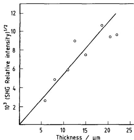
**Figure 5** Variation of the maximum SHG activity found over the film area for PBLG films as a function of film thickness with data showing the square root dependence. Fields during film formation  $\sim 100$  V  $\text{mm}^{-1}$ . Surface variation of film thickness  $< 20\%$
