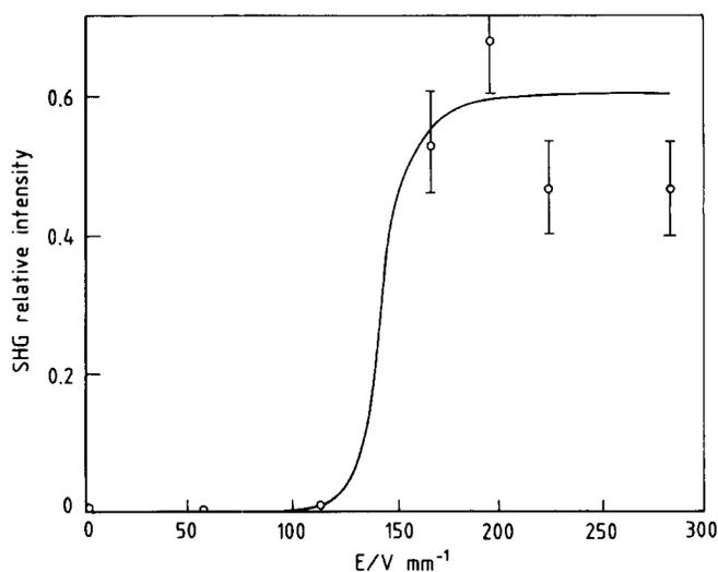
**Figure 3** SHG intensity generated by irradiating  $20 \pm 5 \mu\text{m}$  PHIC films prepared under various aligning fields ( $E$ ). Polarization angle set at  $0^\circ$
