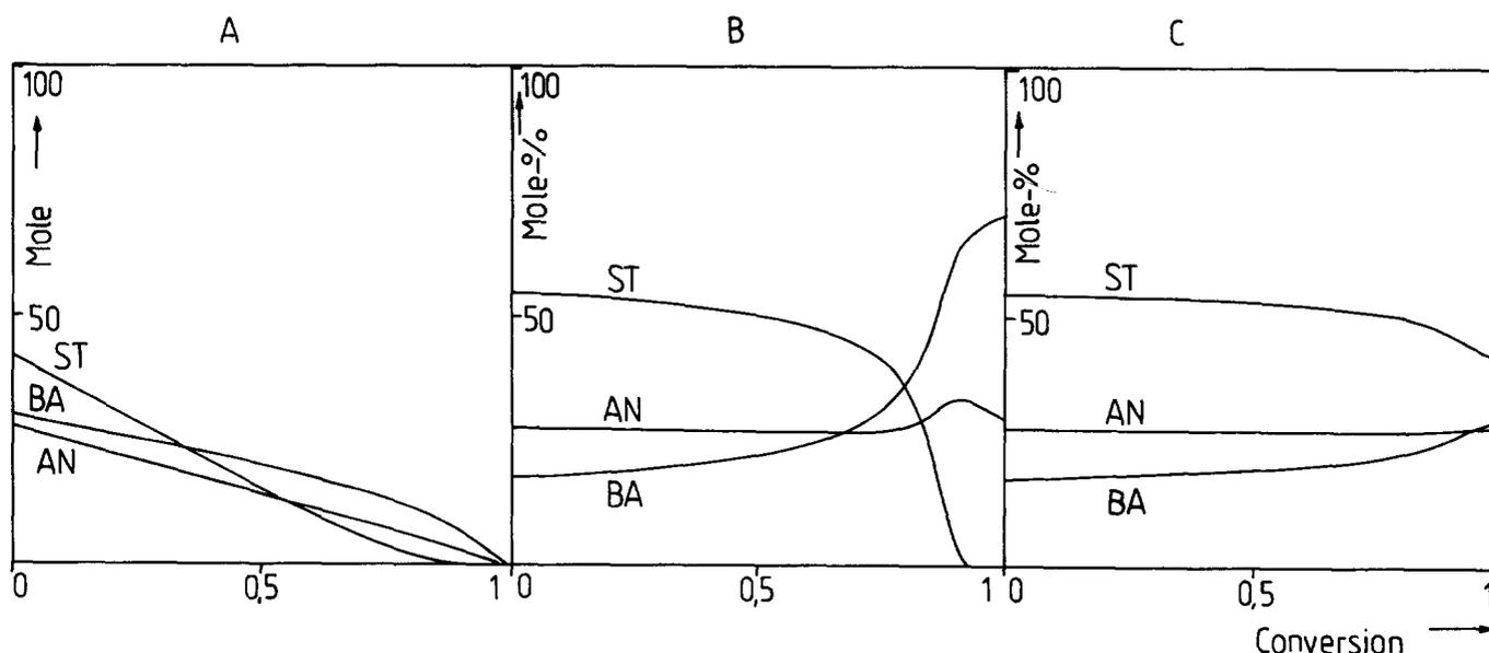
Figure 2 Dependence of the monomer composition (A), differential (B) and integral terpolymer composition (C) on the degree of conversion for the styrene (ST, 42 mol%)/acrylonitrile (AN, 28 mol%)/n-butyl acrylate (BA, 30 mol%) system
