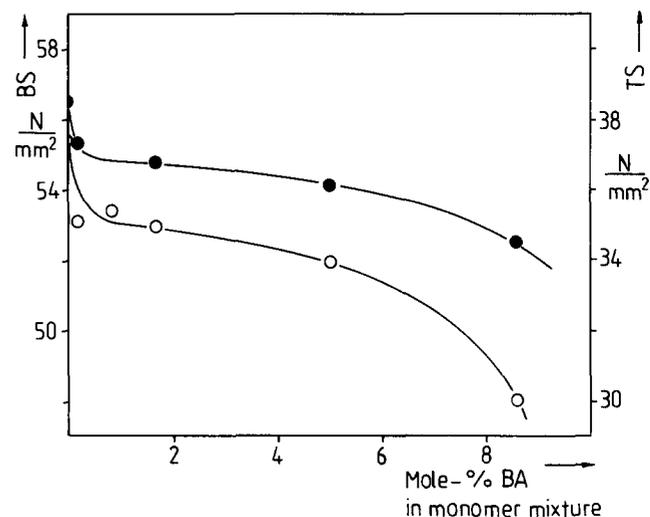
**Figure 6** Dependence of: (○) bending strength (BS); and (●) tensile strength (TS) of the graft polymers on the n-butyl acrylate quantity in the monomer mixture
