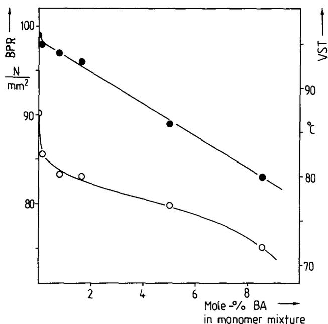
Figure 7 Relationship between: (○) ball-puncture resistance (BPR); and (●) Vicat softening temperature (VST) of the graft polymers and the n-butyl acrylate quantity in the monomer mixture
