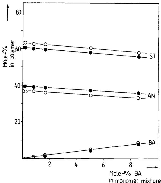
Figure 4 Variation of the polymer composition relative to styrene (ST), acrylonitrile (AN) and n-butyl acrylate (BA) with increasing quantity of n-butyl acrylate in the monomer mixture: (○) experimental; (●) theoretical
