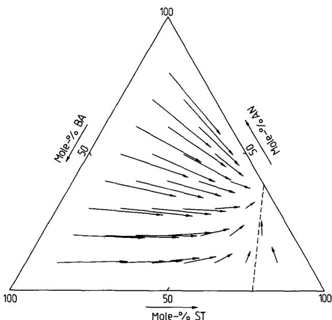
Figure 1 Dependence of terpolymer composition on the composition of the monomer mixture for the styrene (ST)/acrylonitrile (AN)/n-butyl acrylate (BA) system at low degrees of conversion. (---) connecting line between the binary azeotropes
