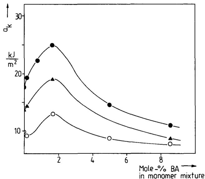
**Figure 5** Relationship between notched impact resistance ( $a_k$ ) of the graft polymers and quantity of n-butyl acrylate (BA) in the monomer mixture. Test temperatures: (●) 293 K; (▲) 273 K; (○) 253 K
