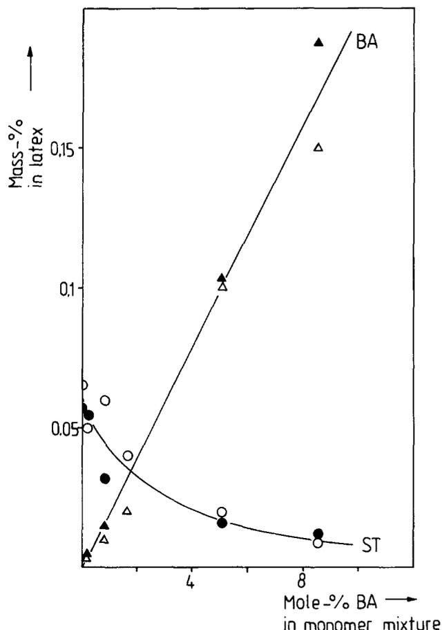
Figure 3 Dependence of the residual styrene content and residual n-butyl acrylate content in the ABS latex on the n-butyl acrylate quantity in the monomer mixture. (○△) Analysis of the ABS latex by gas chromatography; (●▲) steam distillation of the ABS latex and analysis of the organic phase by gas chromatography
