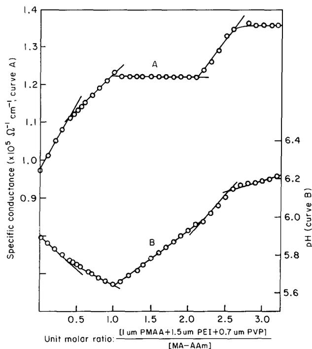
**Figure 5** Variation of conductance and pH with unit mole ratio for the MA-AAm/PMA/PEI/PVP complexation system: (A) conductance; (B) pH
