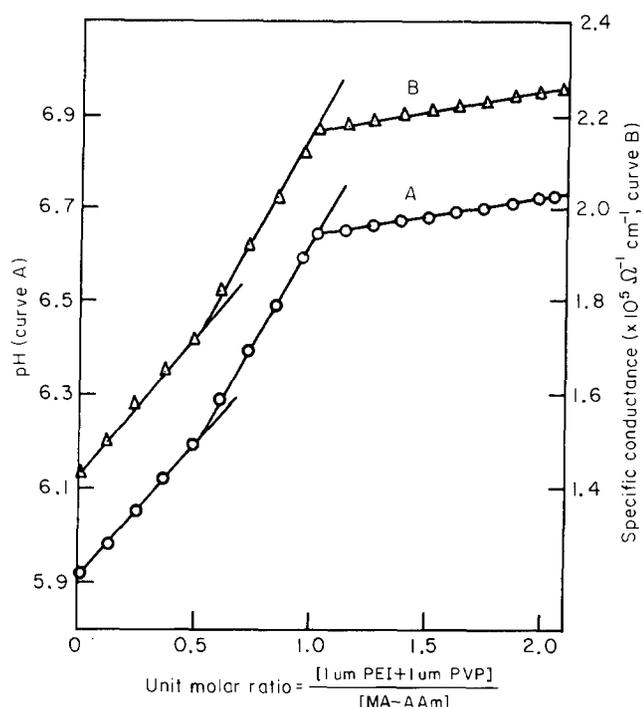
**Figure 4** Variation of pH and conductance with unit mole ratio for the MA-AAm/PEI/PVP complexation system: (A) pH; (B) conductance
