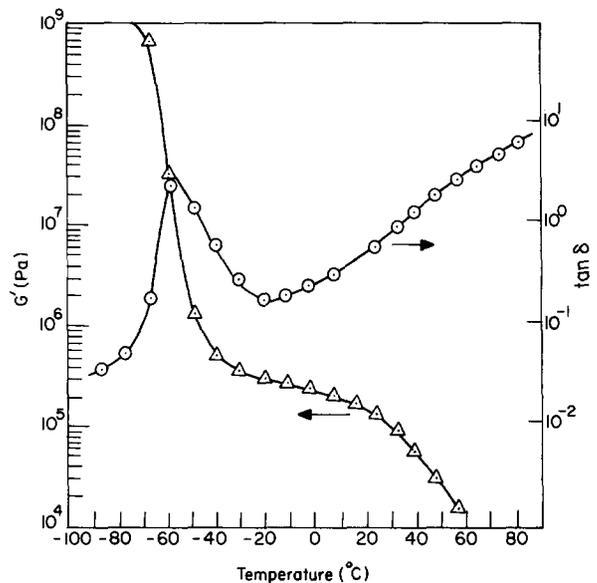
Figure 15 Temperature sweep at  $\omega = 10 \text{ rad s}^{-1}$  of storage modulus  $G'$  (△) and loss tangent  $\tan \delta$  (○) for homopolymer polyisoprene
