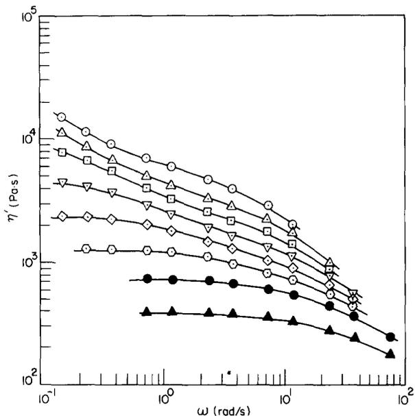
Figure 5 Plots of  $\log \eta'$  versus  $\log \omega$  for K1107 at various temperatures. Symbols are the same as in Figure 1
