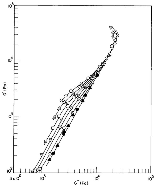
Figure 1 Plots of  $\log G'$  versus  $\log G''$  for K1107 at various temperatures ( $^{\circ}\text{C}$ ): ( $\odot$ ) 160; ( $\triangle$ ) 170; ( $\square$ ) 180; ( $\nabla$ ) 190; ( $\diamond$ ) 200; ( $\circ$ ) 210; ( $\bullet$ ) 220; ( $\blacktriangle$ ) 230
