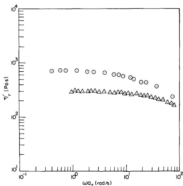
Figure 9 Plots of  $\log \eta'_r$  versus  $\log \omega a_T$  in the disordered state for: (○) K1107; (△) SIS-A. The reference temperature is 220°C
