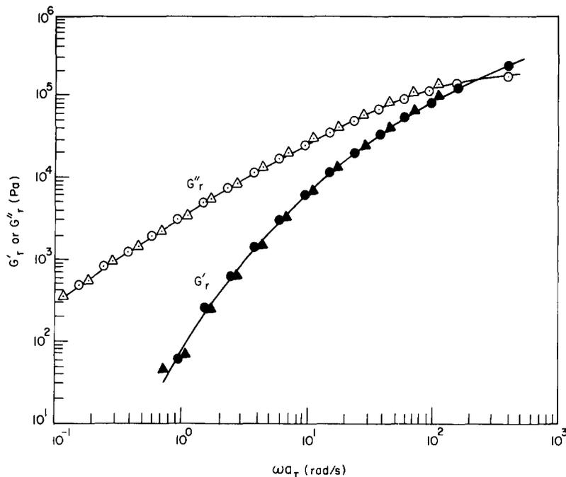
Figure 22 Plots of  $\log G'_r$  (closed symbols) versus  $\log G''_r$  (open symbols) for SIS-C with reference temperature at: ( $\circ$ ,  $\bullet$ ) 105°C; ( $\triangle$ ,  $\blacktriangle$ ) 115°C
