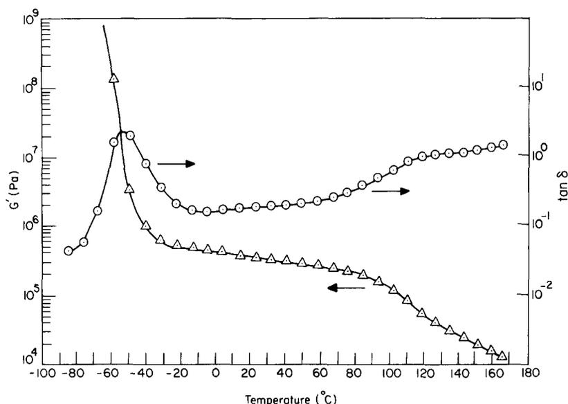
Figure 17 Temperature sweep at  $\omega = 10 \text{ rad s}^{-1}$  of the storage modulus  $G'$  ( $\triangle$ ) and loss tangent  $\tan \delta$  ( $\odot$ ) for SIS-A
