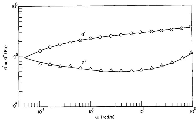
Figure 16 Frequency sweep at  $-20^{\circ}\text{C}$  of the storage modulus  $G'$  ( $\odot$ ) and loss modulus  $G''$  ( $\triangle$ ) for homopolymer polyisoprene
