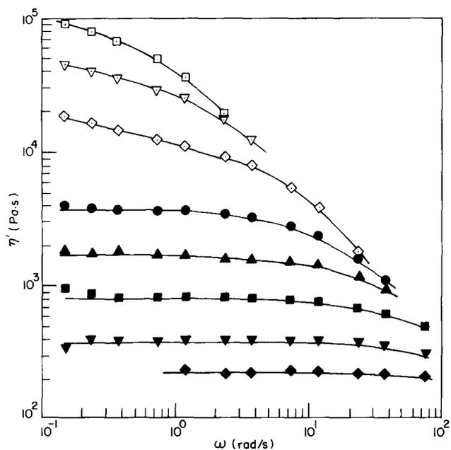
Figure 8 Plots of  $\log \eta'$  versus  $\log \omega$  for SIS-C at various temperatures. Symbols are the same as in Figure 4
