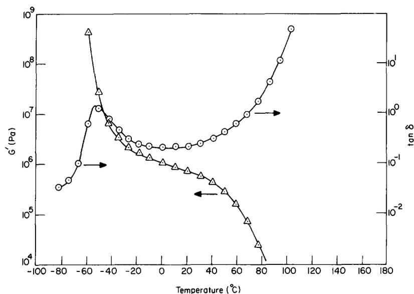
Figure 19 Temperature sweep at  $\omega = 10 \text{ rad s}^{-1}$  of the storage modulus  $G'$  ( $\triangle$ ) and loss tangent  $\tan \delta$  ( $\circ$ ) for SIS-B
