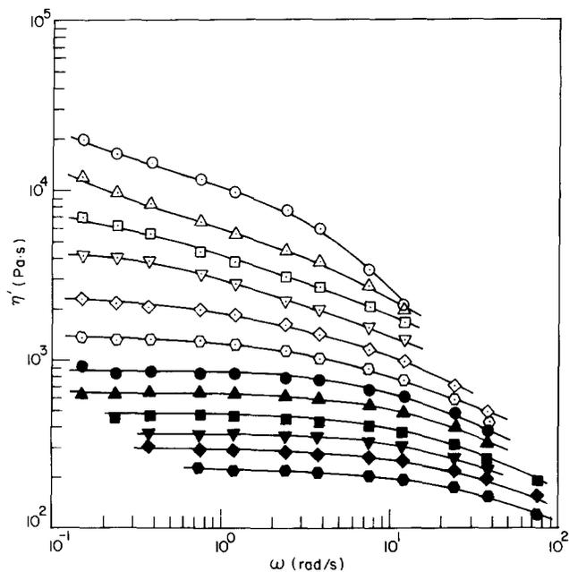
Figure 6 Plots of  $\log \eta'$  versus  $\log \omega$  for SIS-A at various temperatures. Symbols are the same as in Figure 2
