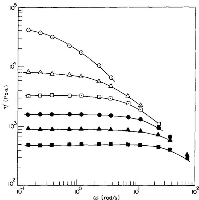
Figure 7 Plots of  $\log \eta'$  versus  $\log \omega$  for SIS-B at various temperatures. Symbols are the same as in Figure 3
