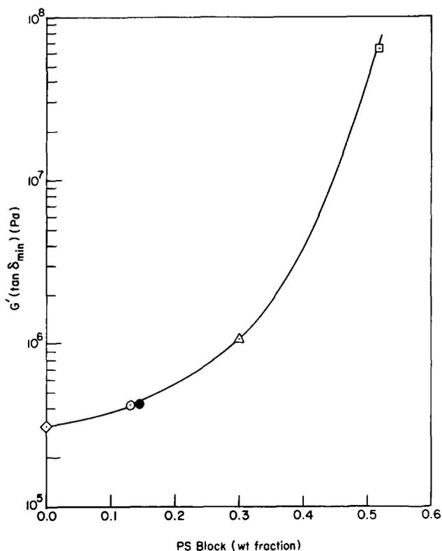
Figure 23 Plots of plateau modulus versus weight fraction of the polystyrene block in microphase-separated SIS triblock copolymer: ( $\circ$ ) SIS-A; ( $\bullet$ ) K1107; ( $\triangle$ ) SIS-B; ( $\square$ ) SIS-C. Also given in the plot is the plateau modulus of homopolymer polyisoprene ( $\diamond$ )
