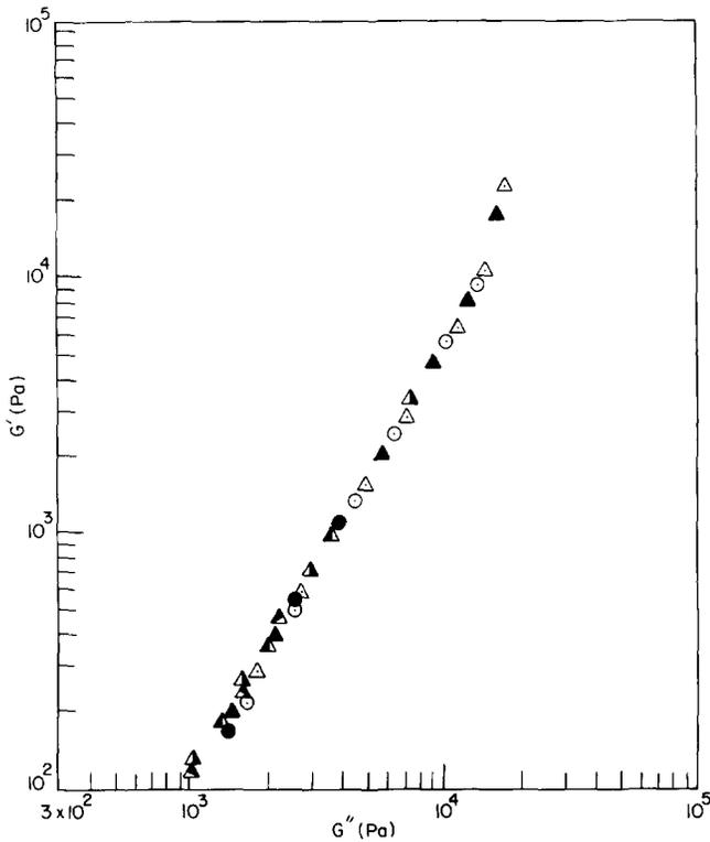
Figure 11 Plots of  $\log G'$  versus  $\log G''$  in the disordered state. K1107 at temperatures ( $^{\circ}\text{C}$ ): ( $\circ$ ) 220; ( $\bullet$ ) 230. SIS-A at temperatures ( $^{\circ}\text{C}$ ): ( $\triangle$ ) 180; ( $\blacktriangle$ ) 190; ( $\blacktriangle$ ) 200; ( $\blacktriangle$ ) 210; ( $\blacktriangle$ ) 220; ( $\blacktriangle$ ) 230
