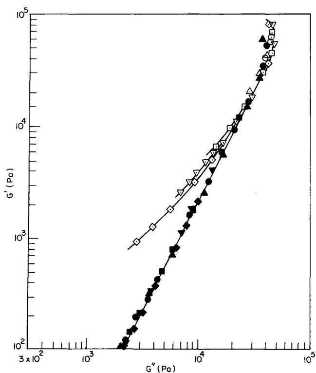
Figure 4 Plots of  $\log G'$  versus  $\log G''$  for SIS-C at various temperatures ( $^{\circ}\text{C}$ ): ( $\odot$ ) 80; ( $\triangle$ ) 85; ( $\square$ ) 90; ( $\nabla$ ) 95; ( $\diamond$ ) 100; ( $\bullet$ ) 105; ( $\blacktriangle$ ) 110; ( $\blacksquare$ ) 115; ( $\blacktriangledown$ ) 120; ( $\blacklozenge$ ) 130
