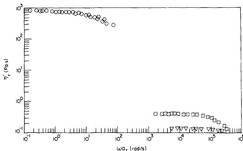
Figure 12 Plots of  $\log \eta'_r$  versus  $\log \omega a_T$  in the disordered state for: ( $\circ$ ) SIS-A; ( $\nabla$ ) SIS-B; ( $\square$ ) SIS-C. The reference temperature is  $180^{\circ}\text{C}$
