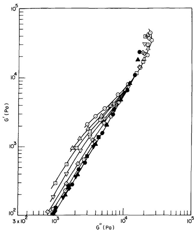
Figure 2 Plots of  $\log G'$  versus  $\log G''$  for SIS-A at various temperatures ( $^{\circ}\text{C}$ ): ( $\odot$ ) 120; ( $\triangle$ ) 130; ( $\square$ ) 140; ( $\nabla$ ) 150; ( $\diamond$ ) 160; ( $\circ$ ) 170; ( $\bullet$ ) 180; ( $\blacktriangle$ ) 190; ( $\blacksquare$ ) 200; ( $\blacktriangledown$ ) 210; ( $\blacklozenge$ ) 220; ( $\bullet$ ) 230
