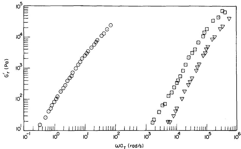
Figure 13 Plots of  $\log G'$  versus  $\log \omega a_T$  in the disordered state for: (○) SIS-A; (▽) SIS-B; (□) SIS-C. The reference temperature is 180°C
