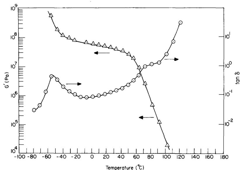
**Figure 21** Temperature sweep at  $\omega = 10 \text{ rad s}^{-1}$  of the storage modulus  $G'$  ( $\triangle$ ) and loss tangent  $\tan \delta$  ( $\circ$ ) for SIS-C
