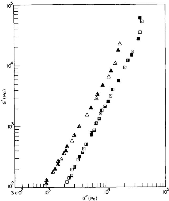
Figure 14 Plots of  $\log G'$  versus  $\log G''$  in the disordered state. SIS-A at temperatures (°C): (△) 180; (▲) 190; (▲) 200; (▲) 210; (▲) 220; (▲) 230. SIS-C at temperatures (°C): (□) 105; (■) 110; (■) 115; (■) 120; (■) 130
