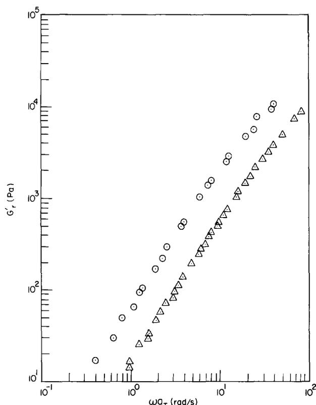
Figure 10 Plots of  $\log G'_r$  versus  $\log \omega a_T$  in the disordered state for: (○) K1107 and (△) SIS-A. The reference temperature is 220°C
