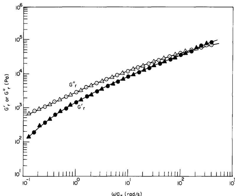
Figure 18 Plots of  $\log G'_r$  (closed symbols) versus  $\log G''_r$  (open symbols) for SIS-A with reference temperature at: ( $\circ$ ,  $\bullet$ ) 180°C; ( $\triangle$ ,  $\blacktriangle$ ) 190°C
