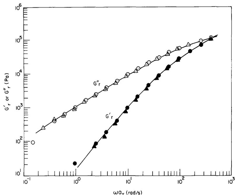
**Figure 20** Plots of  $\log G'_r$  (closed symbols) versus  $\log G''_r$  (open symbols) for SIS-B with reference temperature at: ( $\circ$ ,  $\bullet$ ) 90°C; ( $\triangle$ ,  $\blacktriangle$ ) 100°C
