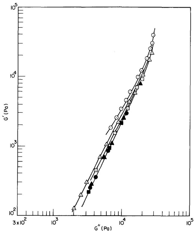
Figure 3 Plots of  $\log G'$  versus  $\log G''$  for SIS-B at various temperatures ( $^{\circ}\text{C}$ ): ( $\odot$ ) 70; ( $\triangle$ ) 80; ( $\square$ ) 85; ( $\bullet$ ) 90; ( $\blacktriangle$ ) 95; ( $\blacksquare$ ) 100
