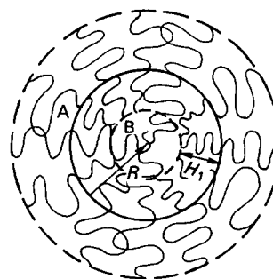
Figure 1 The element of a mixed cylindrical superstructure of a diblock AB copolymer: H_1 , the width of the short B chains sublayer; R , cylinder radius
