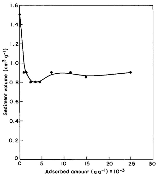
Figure 2 Effect of adsorbed amount on the sediment volume of albite
