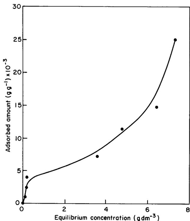
Figure 1 Adsorption isotherm of PMMA on albite ore surface
