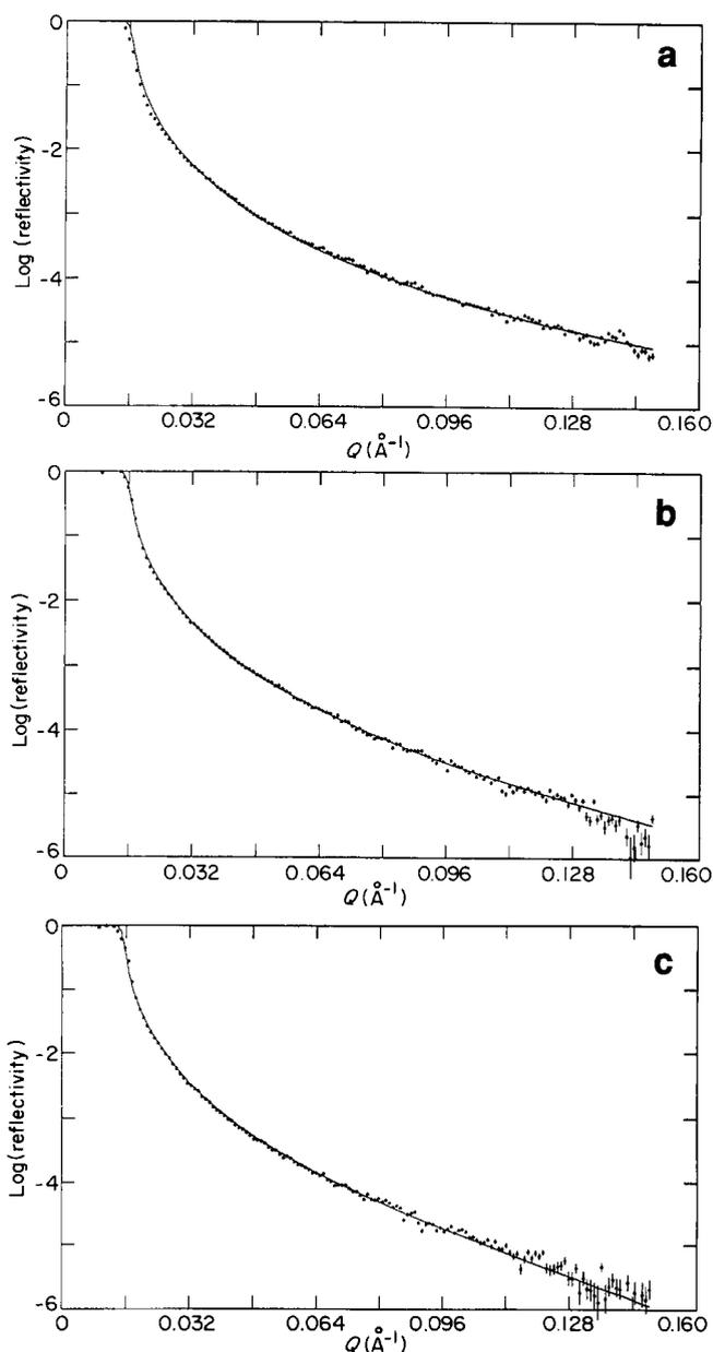
**Figure 1** (a) Reflectivity curve from a deuterated PMMA/silicon interface at  $92.6^\circ\text{C}$ : (●) experimental points; (—) theoretical fit. (b) Same as (a) except the temperature was  $117.8^\circ\text{C}$ . (c) Same as (a) except the temperature was  $144.0^\circ\text{C}$
