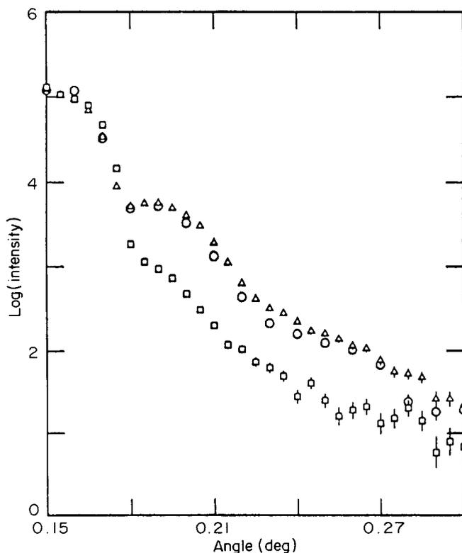
**Figure 3** Results of a transverse scan from a deuterated PMMA/silicon interface at  $Q = 0.014 \text{ \AA}^{-1}$ : (○)  $92.6^\circ\text{C}$ ; (△)  $101.1^\circ\text{C}$ ; (□)  $117.8^\circ\text{C}$
