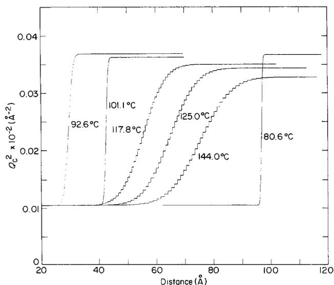
**Figure 2** Density profiles of a deuterated PMMA/silicon interface at six different temperatures during a heating and subsequent cooling cycle. The origin of each profile on the x-axis, or the locations of the interface, was shifted by an arbitrary amount to illustrate the change in the profile shape. The ordinate is  $Q_c^2$  and is linearly related to the local polymer density by a constant factor
