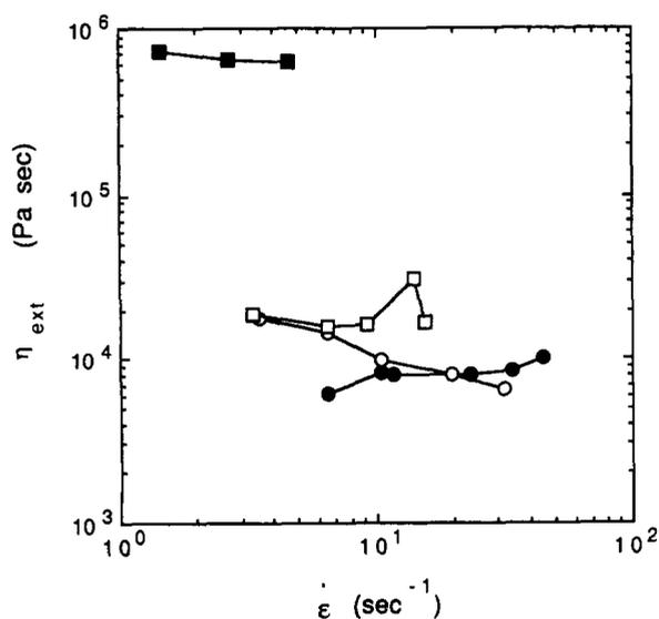
**Figure 3** Estimates of extensional viscosity versus extensional strain rate measured using (i) converging flow analysis for VECTRA at 300°C (○) and HX-2000 at 310°C (□), and (ii) isothermal melt spinning for VECTRA at 300°C (●) and HX-2000 at 300°C (■)
