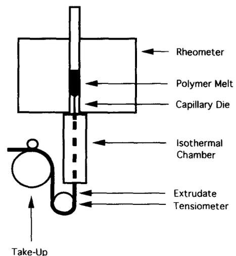
Figure 1 Isothermal melt-spinning apparatus for measuring extensional flow properties
