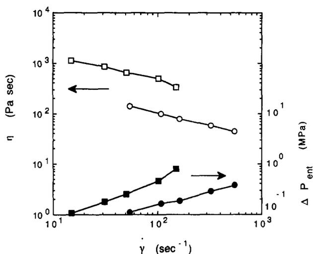
**Figure 2** Shear viscosity of VECTRA at 300°C (○) and HX-2000 at 310°C (□), and entry pressure loss of VECTRA at 300°C (●) and HX-2000 at 310°C (■) versus apparent wall shear rate
