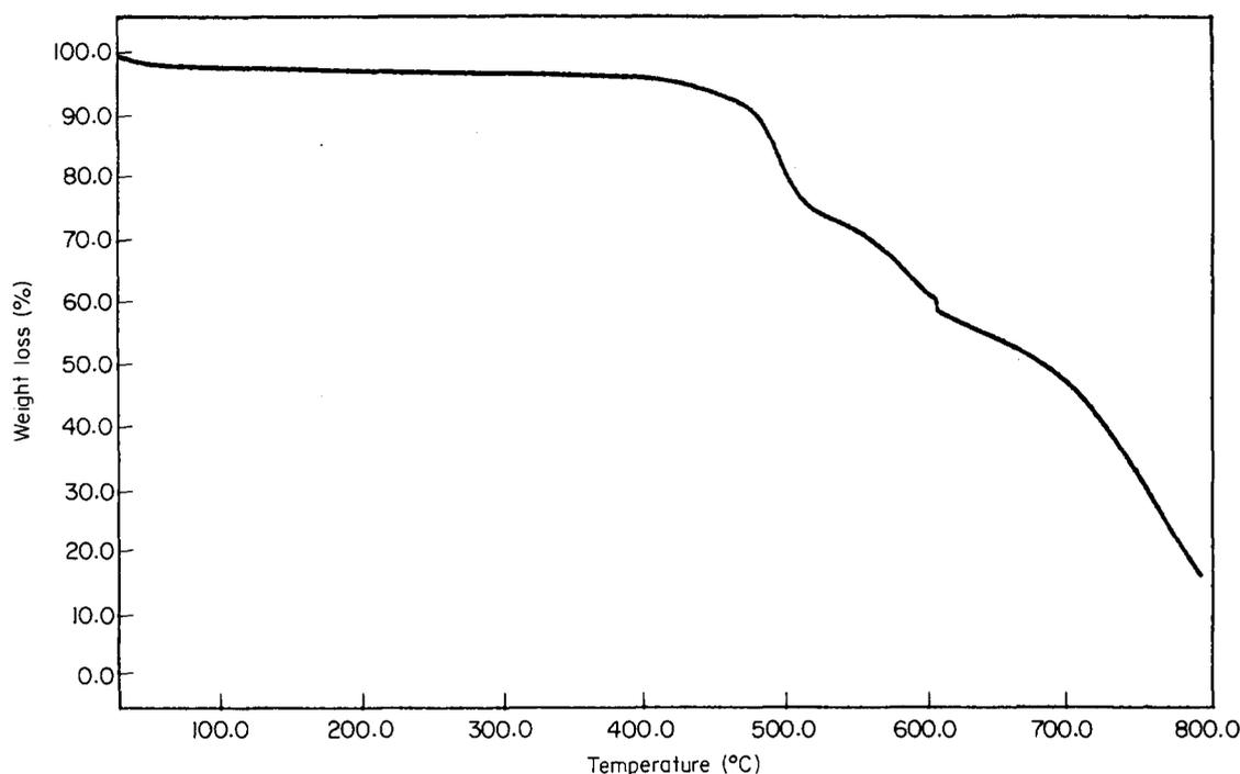
**Figure 1** Thermogravimetric trace of polymer 6 in air flow
