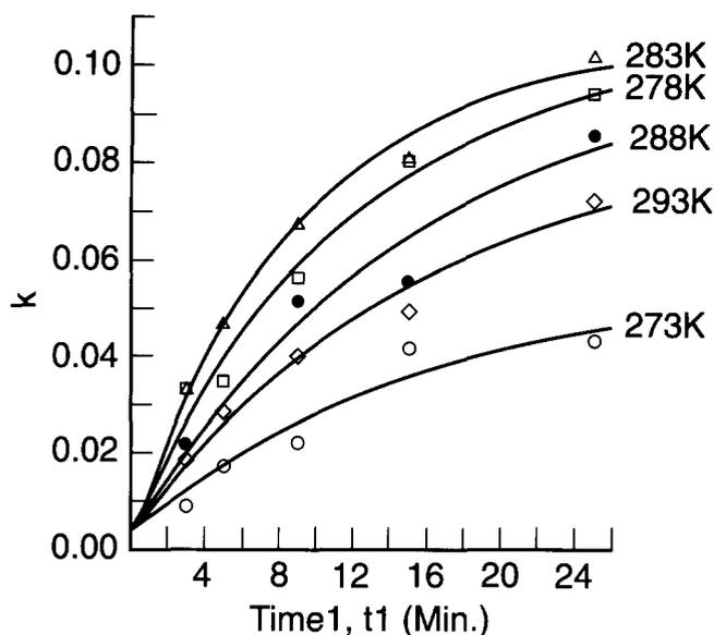
**Figure 7** Plot of rate constant,  $K$ , against nucleation time,  $t_1$ , for 85/15 wt VDC/wt VC copolymer at various nucleation temperatures: (○) 273 K, (□) 278 K, (△) 283 K, (●) 288 K and (◇) 293 K crystallized at 313 K
