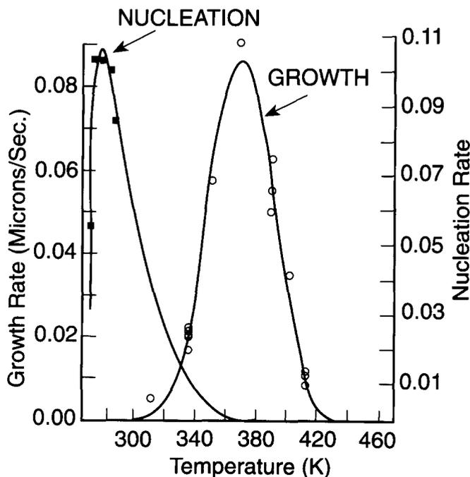
**Figure 8** Plot of growth rate and nucleation rate against temperature for 85/15 wt VDC/wt VC copolymer. Equation (14) was fit to the nucleation data:  $B = 370 \text{ cal mol}^{-1}$  and  $k_n = 616 \text{ K}$
