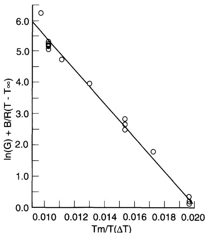
**Figure 3** Plot of  $\ln(G) + B/R(T - T_\infty)$  against  $T_m/T(\Delta T)$  for 85/15 wt VDC/wt VC for the case  $B = 1.69 \text{ kcal mol}^{-1}$ ,  $T_\infty = T_g - 30 \text{ K}$ ,  $T_m = 471 \text{ K}$ ,  $K_g = 499 \text{ K}$  and  $G$  measured in  $\mu\text{m}/\text{min}$
