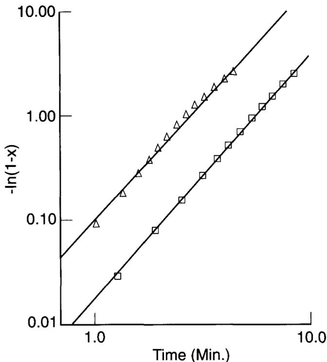
**Figure 5** Plot of  $\log[-\ln(1-X)]$  against  $\log(t-t_1)$  for 85/15 wt VDC/wt VC copolymer at two different nucleation conditions: ( $\square$ )  $T_1 = 293$  K and  $t_1 = 3$  min and ( $\triangle$ )  $T_1 = 283$  K and  $t_1 = 25$  min
