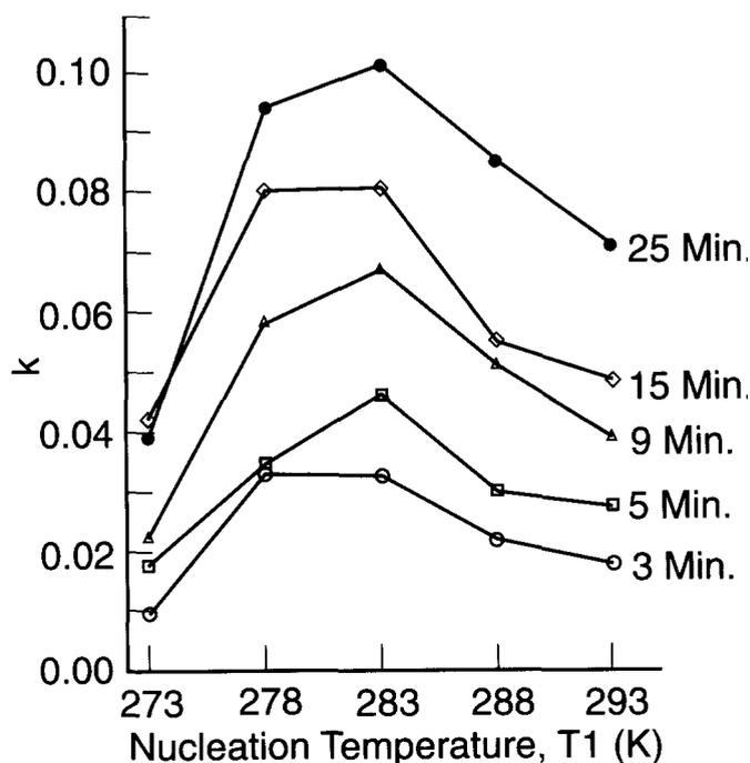
**Figure 6** Plot of rate constant,  $K$ , against nucleation temperature,  $T_1$  (K) for 85/15 wt VDC/wt VC copolymer at various nucleation times: ( $\circ$ ) 3 min, ( $\square$ ) 5 min, ( $\triangle$ ) 9 min, ( $\diamond$ ) 15 min and ( $\bullet$ ) 25 min crystallized at 313 K
