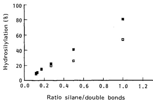
**Figure 3** Hydrosilylation yield (□, experimental; ■, theoretical) as a function of the ratio silane/double bonds, assuming for the theoretical values that the reaction is selective to the 1,2-polybutadiene units
