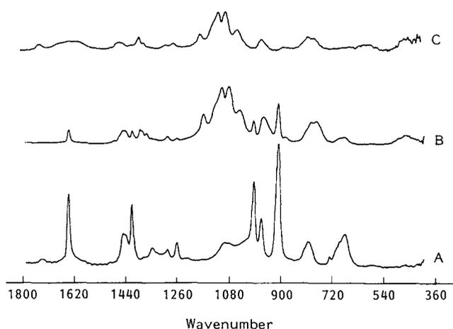
Figure 1 Infrared spectra of polybutadiene before (A) and after hydrosilylation at 19% (B) or 54% (C)
