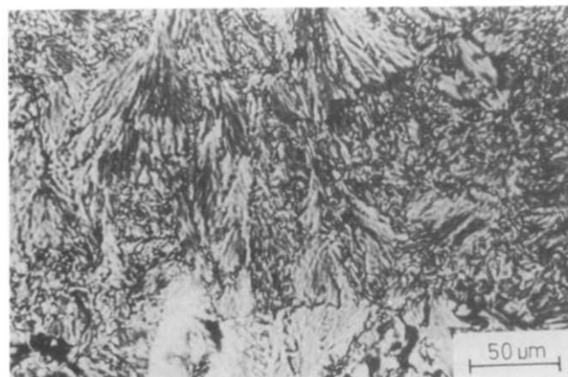
Figure 5 Optical micrograph (crossed polarizers) of the texture of the crystal solvate in the LC+CS region of Figure 3
