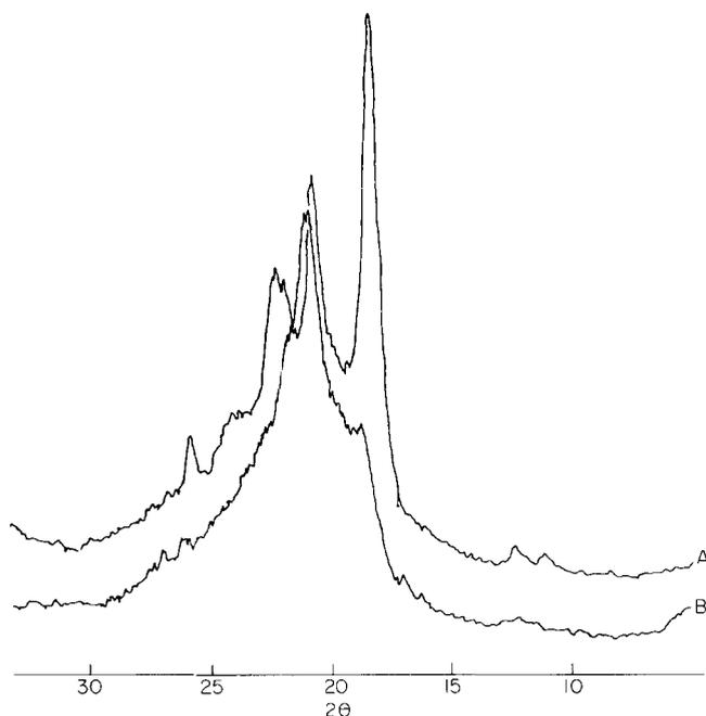
**Figure 4** X-ray diffraction diagrams for poly(amide-ester) film POLEA 3612: A, after degradation; B, before degradation
