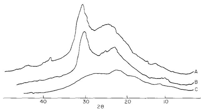
Figure 3 X-ray diffraction diagrams for poly(amide-ester) film POLEA 366/26: A, before in vitro test; B, after 10 days; C, after 30 days
