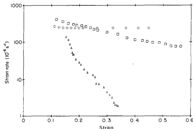
Figure 2 Sherby-Dorn plots derived from the data in Figure 1. O, HP; □, CP1; △, CP2
