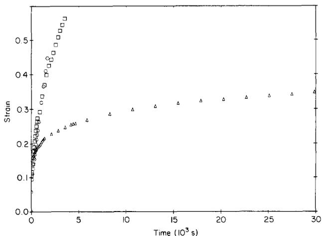
Figure 1 Room temperature creep data for samples of the three materials drawn to their natural draw ratio. Stress levels are as shown in Table 2. O, HP; □, CP1; △, CP2
