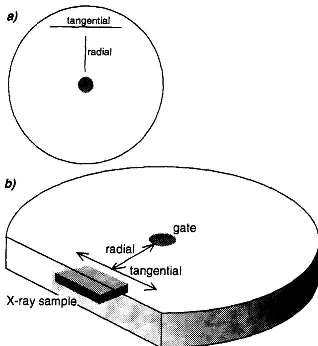
**Figure 1** Diagram of disc: (a) definition of radial and tangential directions; (b) location from which samples were taken. (Non-uniform scale: disc diameter 150 mm, thickness 4 mm; X-ray sample thickness 0.2 mm)
