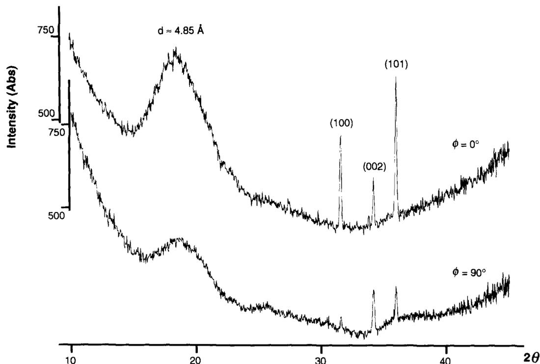
Figure 3 X-ray diffractograms of the EPDM sample at the azimuthal angles  $\phi = 0$  and  $\phi = 90^\circ$
