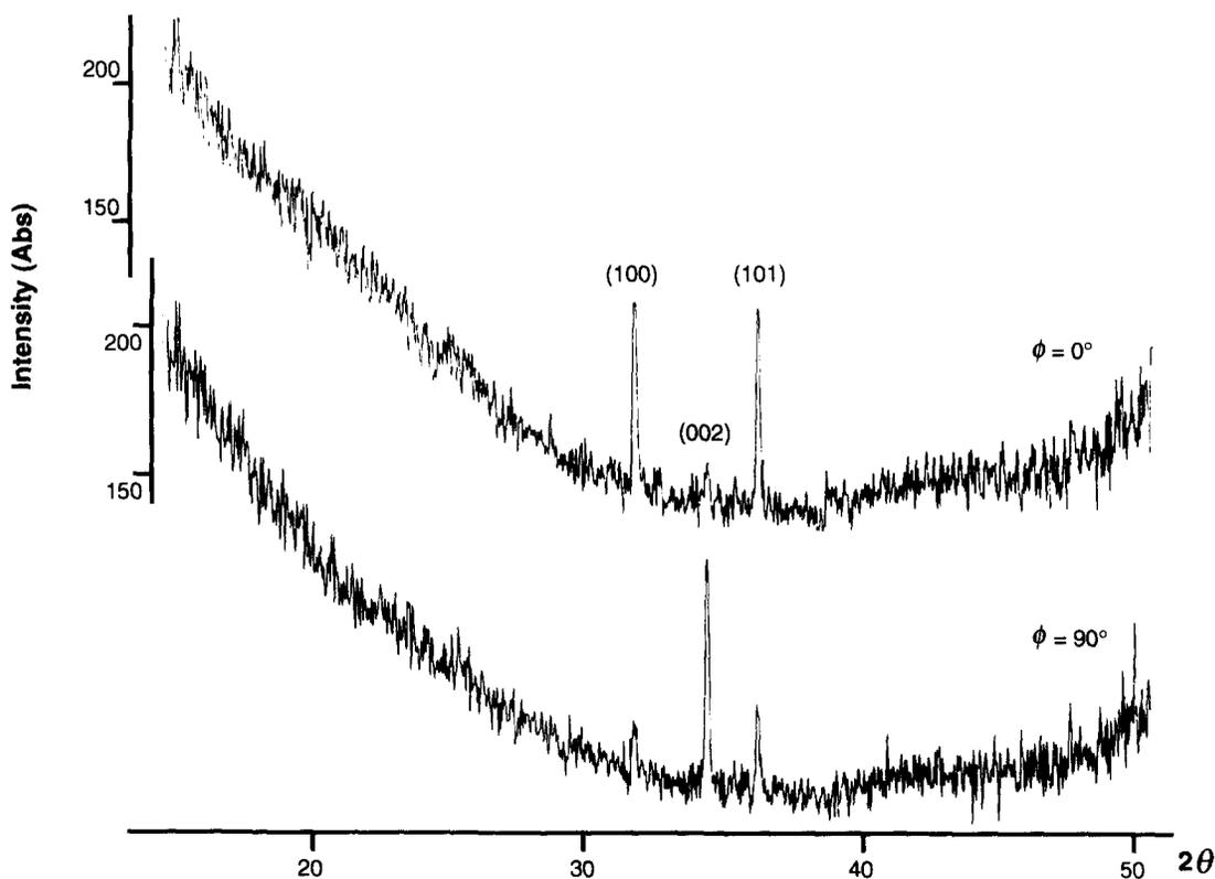
Figure 4 X-ray diffractograms of the SBR sample at the azimuthal angles  $\phi = 0$  and  $\phi = 90^\circ$
