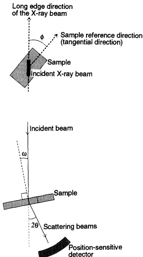
**Figure 2** Diagrams showing the position of sample during the scattering measurements
