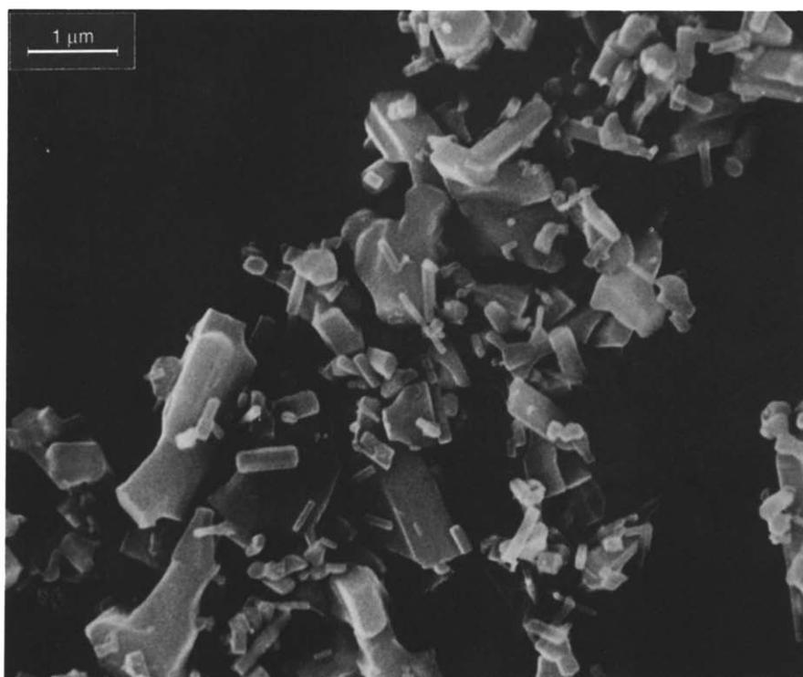
Figure 5 Scanning electron micrograph of the zinc oxide
