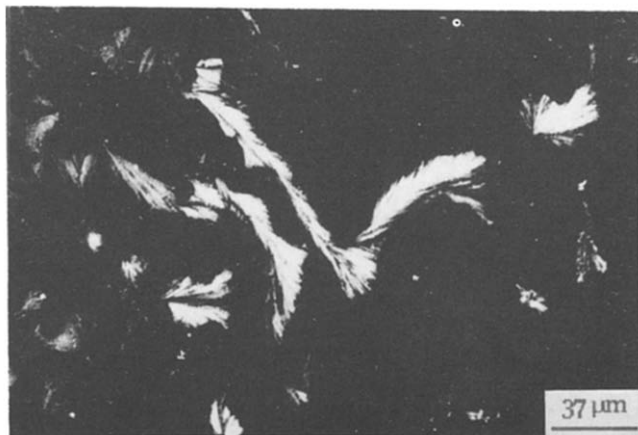
Figure 5 Preferentially developed edges of PEEK crystallized at 315°C
