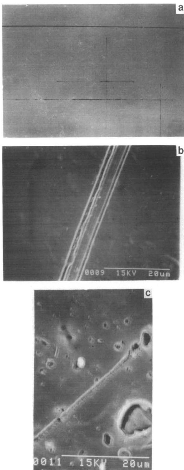
**Figure 1** Scanning electron micrographs of ungrafted and grafted cellulose acetate films. (a) Ungrafted film; (b) acrylamide grafted film with simultaneous irradiation; (c) acrylamide grafted film with preirradiation process (magnification 2000 ×)
