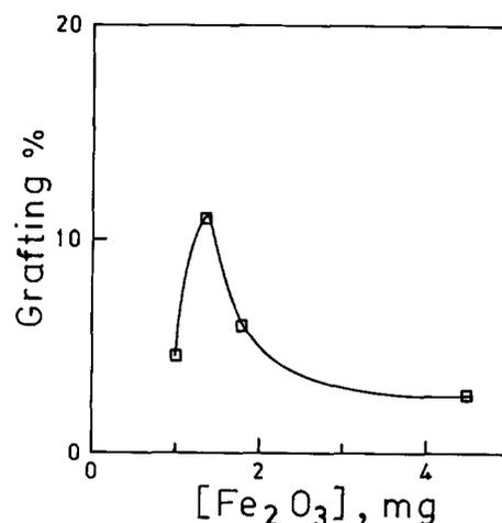
**Figure 2** Variation of degree of grafting with concentration of colloidal  $\text{Fe}_2\text{O}_3$ . ( $[\text{acrylamide}] = 1 \text{ M}$ )
