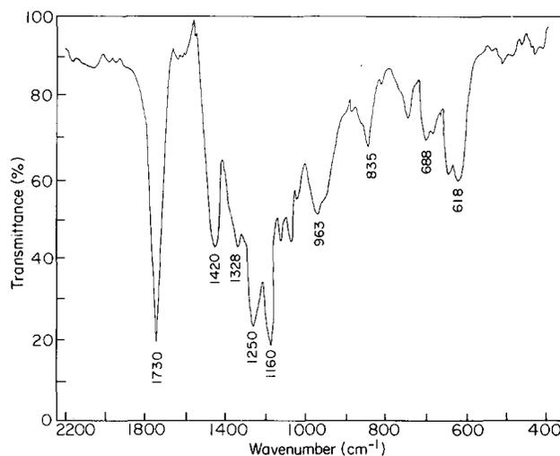
**Figure 6** FTi.r. spectrum of the graft copolymer
