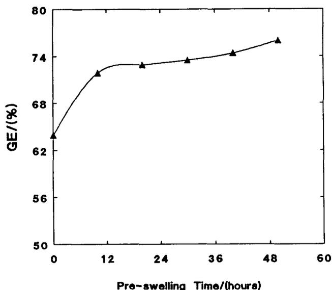
**Figure 1** Effect of pre-swelling time on grafting efficiency. BA/PVC = 40/60; initiator concentration, 0.2%; reaction conditions, 50°C, 5 h
