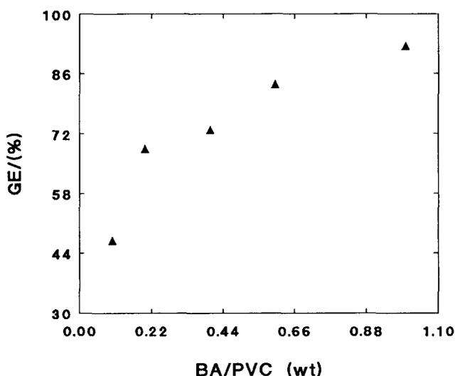
**Figure 2** Effect of BA/PVC ratio on grafting efficiency. Initiator concentration, 0.2 wt%; pre-swelling time, 20 h; reaction conditions, 50°C, 5 h
