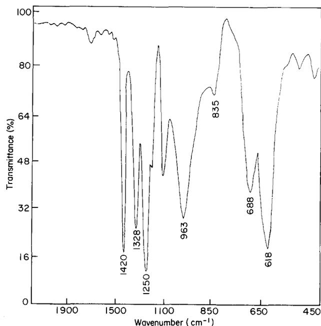
**Figure 4** FTi.r. spectrum of PVC
