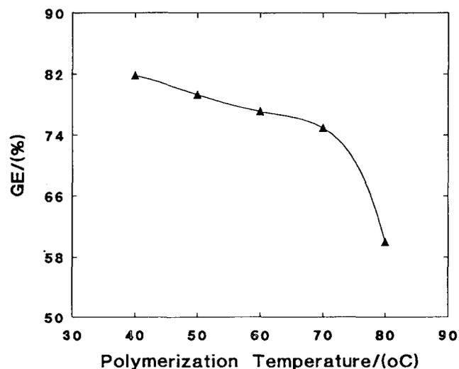
**Figure 3** Effect of temperature on grafting efficiency. BA/PVC = 30/70; initiator concentration, 0.2 wt%
