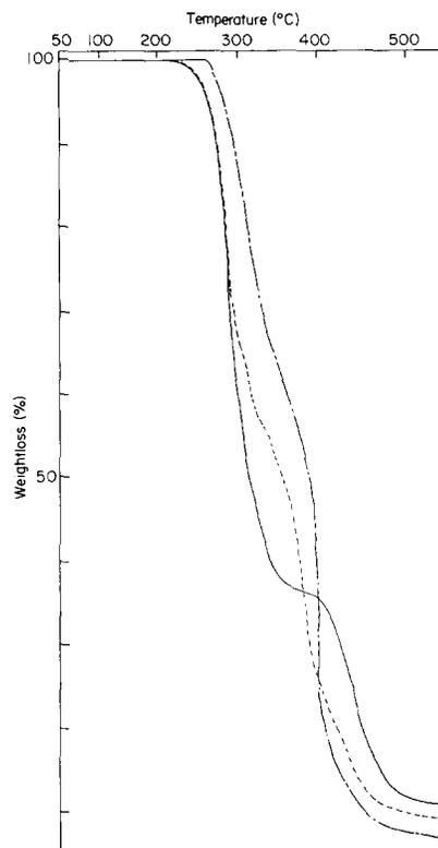
Figure 9 Results of thermogravimetric analysis (in  $\text{N}_2$ ): —, PVC; ---, PVC/PBA (80/20) blend; - · - ·, resultant graft copolymer
