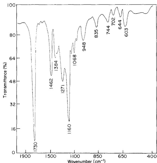
Figure 8 FTIR spectrum of the PBA homopolymer produced in graft copolymerization
