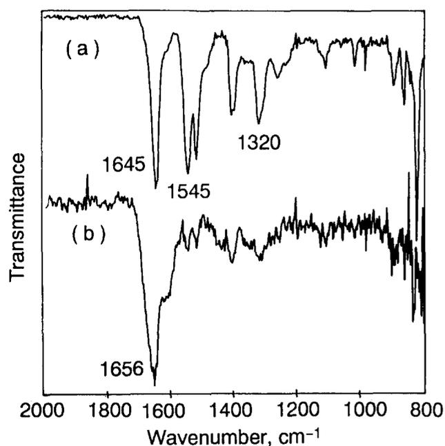
**Figure 2** A.T.R.-FTi.r. spectra of (a) the virgin aramid fibre and (b) the PAAm-grafted aramid fibre (30 s plasma exposure, 10 wt% AAm solution, 30°C and 50 min u.v. irradiation)
