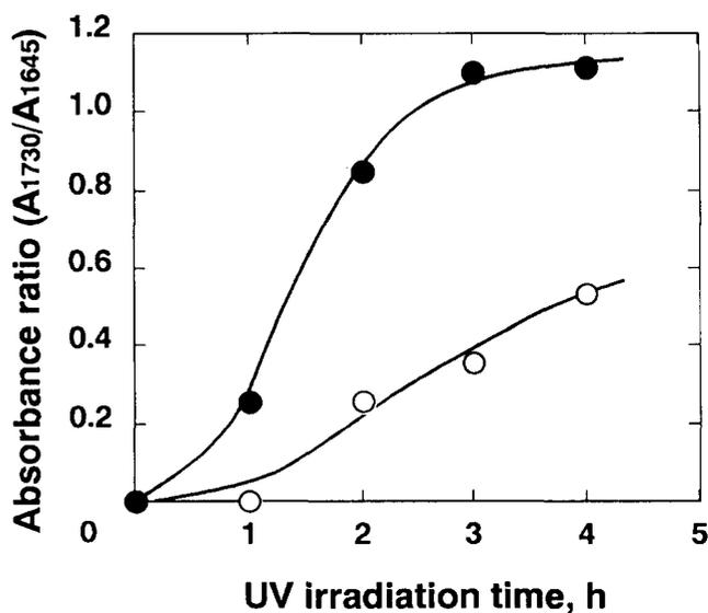
Figure 7 Changes in the absorbance ratio of the carbonyl peak at  $1730\text{ cm}^{-1}$  to the amide peak at  $1645\text{ cm}^{-1}$  for the aramid fibre grafted with PGMA by u.v. irradiation for different times after plasma treatment for 60 s: (○) 10 vol% GMA; (●) 20 vol% GMA
