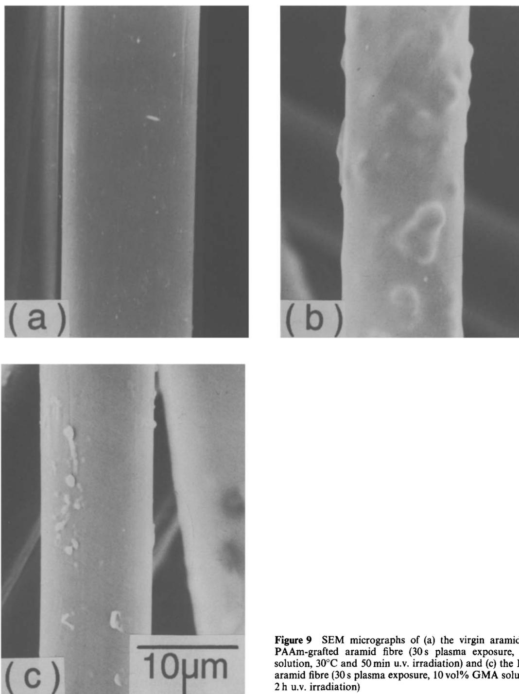
**Figure 9** SEM micrographs of (a) the virgin aramid fibre, (b) the PAAm-grafted aramid fibre (30 s plasma exposure, 10 wt% AAm solution, 30°C and 50 min u.v. irradiation) and (c) the PGMA-grafted aramid fibre (30 s plasma exposure, 10 vol% GMA solution, 30°C and 2 h u.v. irradiation)
