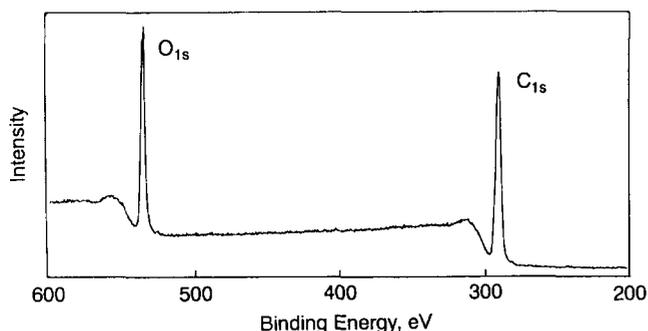
Figure 5 XPS spectrum of the PGMA-grafted aramid fibre (30 s plasma exposure, 10 vol% GMA solution, 30°C and 2 h u.v. irradiation)
