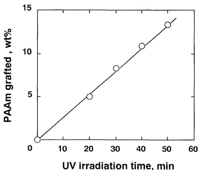
Figure 1 Weight increase by AAm graft polymerization induced by u.v. irradiation at 30°C in 10 wt% AAm solution onto the aramid fibre pre-exposed to Ar plasma for 30 s
