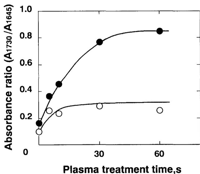
Figure 6 Changes in the absorbance ratio of the carbonyl peak at  $1730\text{ cm}^{-1}$  to the amide peak at  $1645\text{ cm}^{-1}$  for the aramid fibre grafted with PGMA by u.v. irradiation for 2 h after plasma treatment for different times: (○) 10 vol% GMA; (●) 20 vol% GMA
