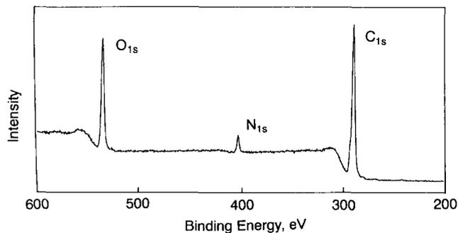
Figure 8 XPS spectrum of the PGMA-grafted aramid fibre after reaction with propylamine for 4 h (graft polymerization: 30 s plasma exposure, 10 vol% GMA solution, 30°C and 2 h u.v. irradiation)
