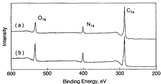
**Figure 3** XPS spectra of (a) the virgin aramid fibre and (b) the PAAm-grafted aramid fibre (30 s plasma exposure, 10 wt% AAm solution, 30°C and 50 min u.v. irradiation)
