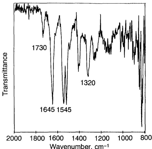
**Figure 4** A.T.R.-FTi.r. spectrum of the PGMA-grafted aramid fibre (30 s plasma exposure, 10 vol% GMA solution, 30°C and 2 h u.v. irradiation)
