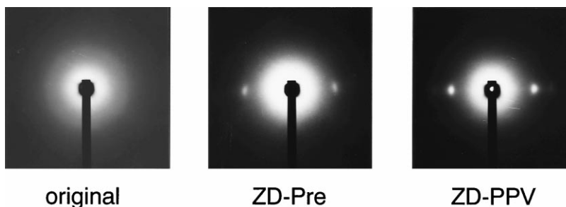
Fig. 4. Wide angle X-ray diffraction photographs of the original, ZD-Pre and ZD-PPV films.
