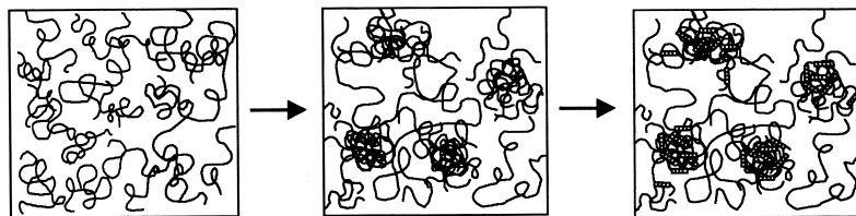
(a) Polymer solution (b) Spinodal decomposition (c) Gelation/crystallization
