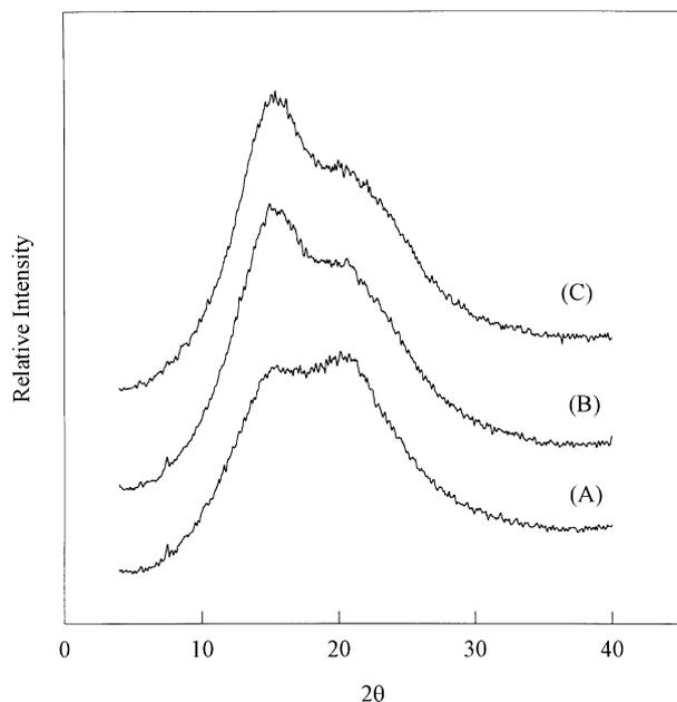
Fig. 1. Wide angle X-ray diffractograms of: (A) PPO:GFRsPS(50:50); (B) 67:33; (C) 75:25.
