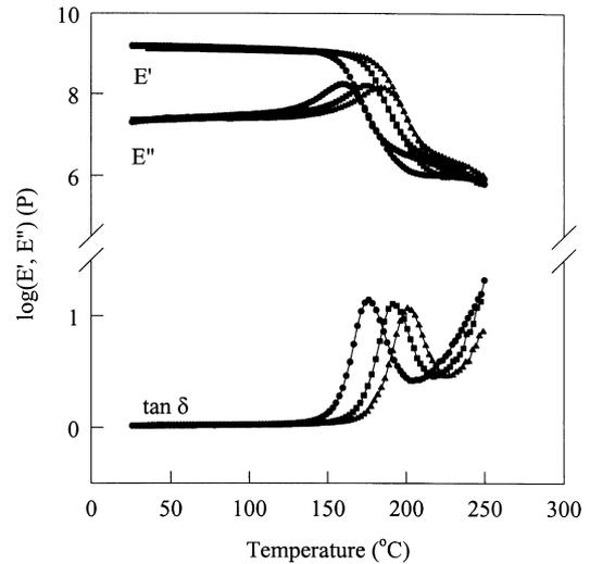
Fig. 2. Dynamic mechanical thermal spectrum of PPO/GFRsPS blends. (●) PPO/GFRsPS (50:50) (■) 67:33 (▲) 75:25.
