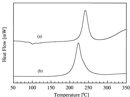
Fig. 4. DSC thermograms of monofunctional benzoxazine monomers: (a) Ph-apc and (b) Ph-apa.
