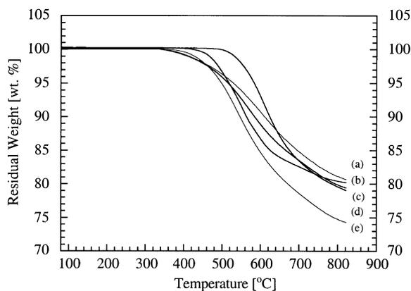
Fig. 6. TGA curves of polybenzoxazine from: (a) HQ-apa; (b) BZ-apa; (c) Ph-apc; (d) Ph-apa and (e) BA-apa, polymerized for 3 h at 190°C in air.
