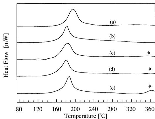
Fig. 5. DSC thermograms of bifunctional benzoxazine monomers: (a) BP-apa; (b) BZ-apa; (c) HQ-apa; (d) BS-apa and (e) BA-apa.
