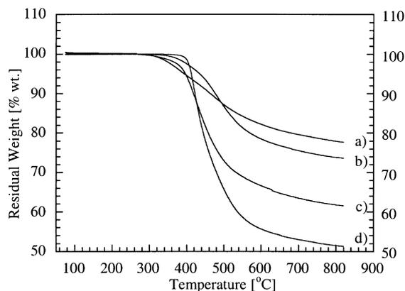
Fig. 7. TGA curves of polybenzoxazines from: (a) HQ-apa; (b) Ph-apa; (c) BZ-apa; and (d) BA-apa, polymerized for 3 h in  $N_2$ .
