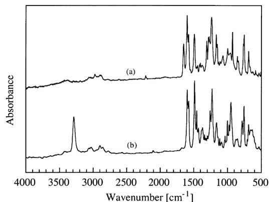
Fig. 1. Fourier transform infrared spectra of monofunctional benzoxazine monomers: (a) Ph-apc and (b) Ph-apa.
