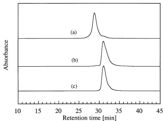
Fig. 2. SEC chromatograms of benzoxazine monomers: (a) BZ-apa; (b) HQ-apa and (c) Ph-apa.
