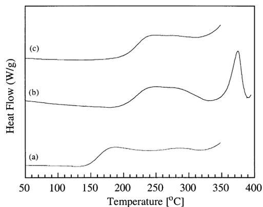
Fig. 8. DSC thermograms of BA-apa, polymerized for 3 h in  $N_2$ : (a) 160°C; (b) 180°C and (c) 190°C.
