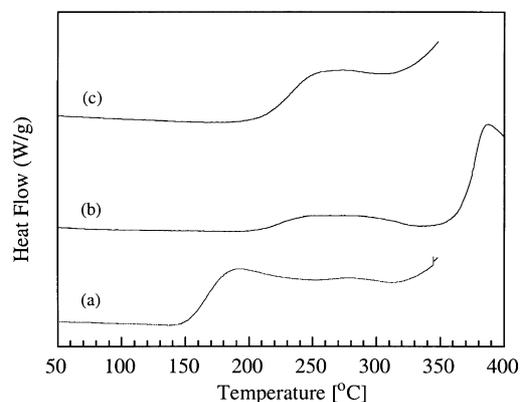
Fig. 9. DSC thermograms of BA-apa, polymerized for 3 h in air: (a) 160°C; (b) 180°C and (c) 190°C.
