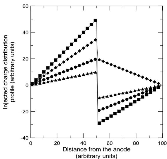
Fig. 7. Idealized profiles of charge injected from electrodes. ▲ ( $T_1$ ); ● ( $T_2$ ); ■ ( $T_3$ ); ◆ ( $T_4$ ).  $T_1 < T_2 < T_3 < T_4$ . The profile corresponding to  $T_4$  shows a sharp increase of charge injection from the anode and positive carriers diffusion through the sample.
