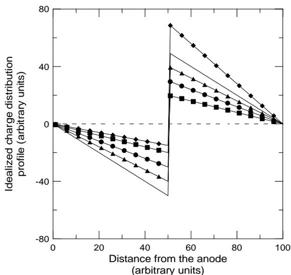
Fig. 8. Profiles resulting from the addition of the idealized profiles of Fig. 7 to a polar symmetric profile (continuous line without symbols). The symbols are as indicated in Fig. 7.
