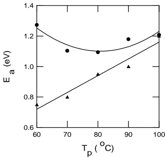
Fig. 4. Activation energies as a function of the polarization temperature. Calculation method: ▲ initial slope; ● curve fitting to the Bucci-Fieschi equation.
