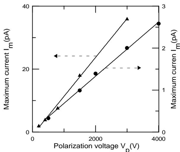
Fig. 6. Maximum current as a function of the applied voltage. Polarization parameters:  $t_p = 30$  min;  $T_p$ : ● (60°C); ▲ (112°C).
