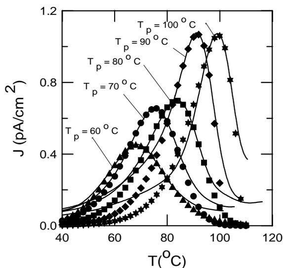
Fig. 2. TSDC of windowing polarized PMMA electrets. Polarization parameters:  $t_p = 2$  min,  $V_p = 2$  kV,  $T_p$  as indicated in the figure, polarization window width  $10^\circ\text{C}$ . (Continuous lines: experimental curves; Symbols: calculated values.)
