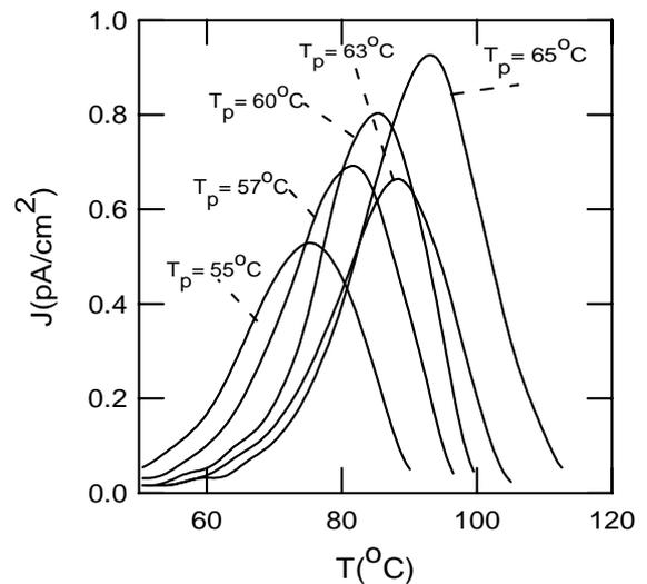
Fig. 5. TSDC of PMMA electrets polarized by a windowing method. Polarization parameters:  $t_p = 2$  min,  $V_p = 4$  kV,  $T_p$  as indicated in the figure, polarization window width 0°C.
