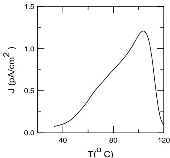
Fig. 1. TSDC of a conventionally polarized PMMA electret. Polarization parameters:  $T_p = 100^\circ\text{C}$ ,  $t_p = 2$  min,  $V_p = 2$  kV.
