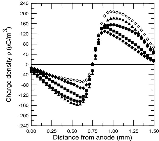
Fig. 3. Space charge distribution profiles of the electrets whose discharges are represented in Fig. 2. They were measured before the stimulated depolarization. Polarization temperatures: ▲ (60°C); ● (70°C); ■ (80°C); ◆ (90°C); ◇ (100°C).
