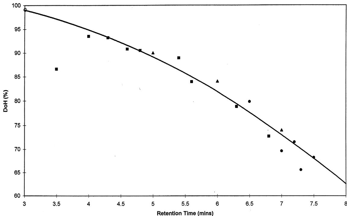
Fig. 2. Calibration curve of DoH vs. retention time for PVOH: (■) PLS3 series fractions; (▲) PLS3 series whole polymers; (●) B72 fractions; (○) 100% hydrolysed polymer.
