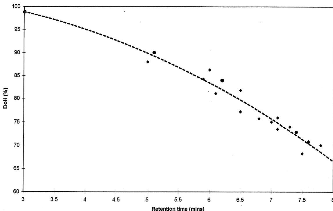
Fig. 3. Calibration results for PVOH: (◆) PLS5 series fractions; (●) PLS5 series whole polymers; (○) 100% hydrolysed polymer; (---) interpolated calibration curve from Fig. 2.
