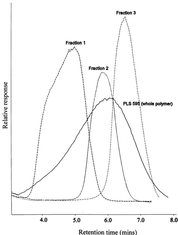
Fig. 1. Chromatograms from reversed phase HPLC of PVOH sample PLS595 and reinjected fractions isolated from this PVOH sample.
