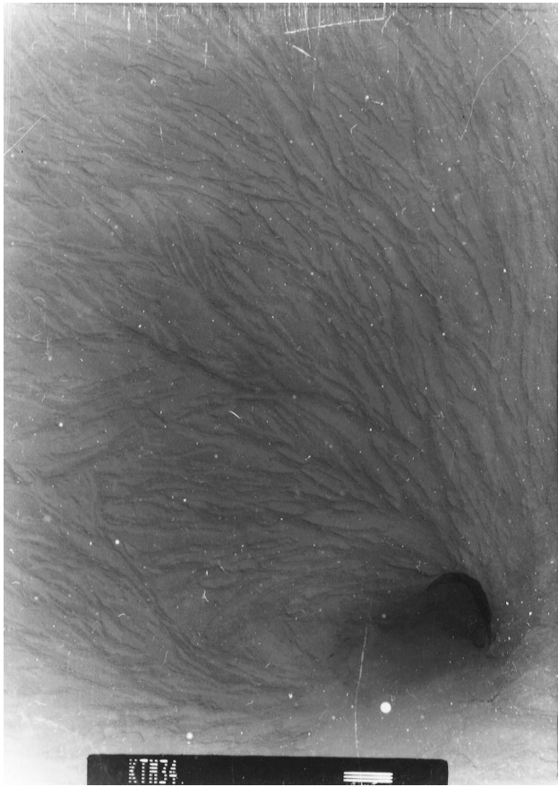
Fig. 5. TEM observations of PEEK edge-on lamellar morphology in spherulites crystallized from the glassy state at 220°C for 24 h. After the melting of the thinner lamellae. Scale bar is 200 nm.
